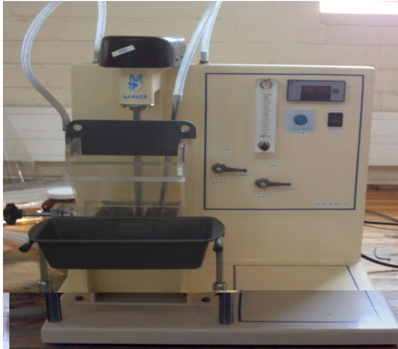
Figure 13: Image of the Leeds flotation cell used in the batch flotation tests
