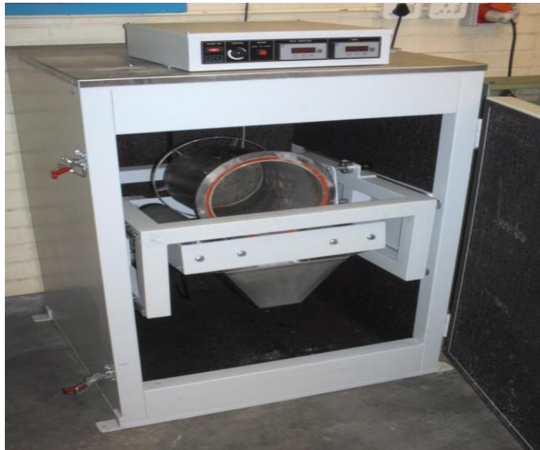
Figure 12: Image of the rod mill used for grinding the ore samples
