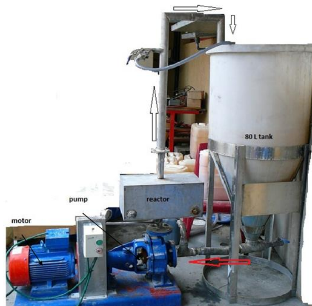
Figure 3-5: Set-up of jet loop pilot plant (Madzivire, 2012)
