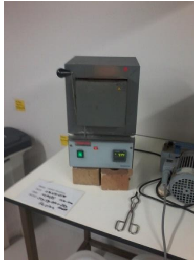
Figure 3-2: Furnace used for alkali fusion of fly ash
