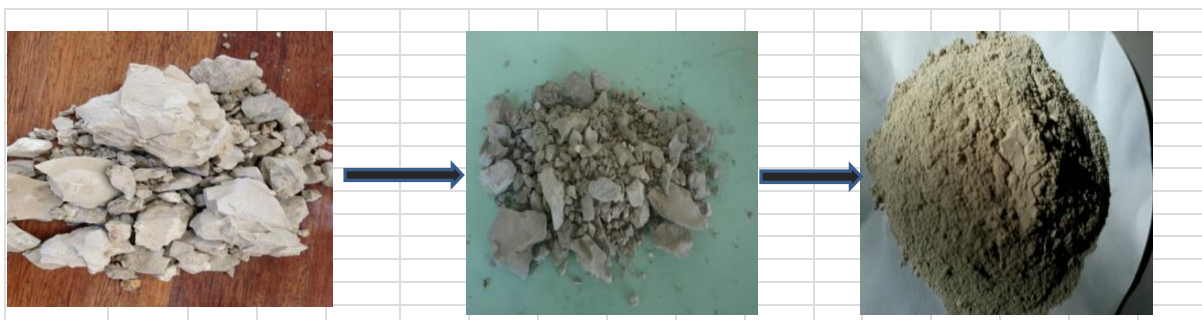
Figure 7. 29: Non-modified natural (Raw) bentonite before and after crushing and milling (Prior Catalytic reaction and beneficiation)
