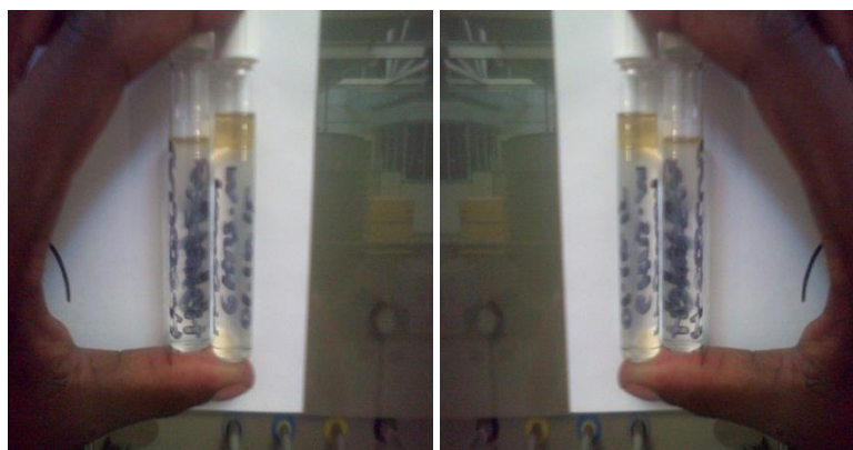
Figure 4.34: Comparison of H-ZeoClay and H-ZeoCOM by physical visibility of liquid product (Closest to the centre: H-ZeoCOM and far end from the centre, H-ZeoClay).
