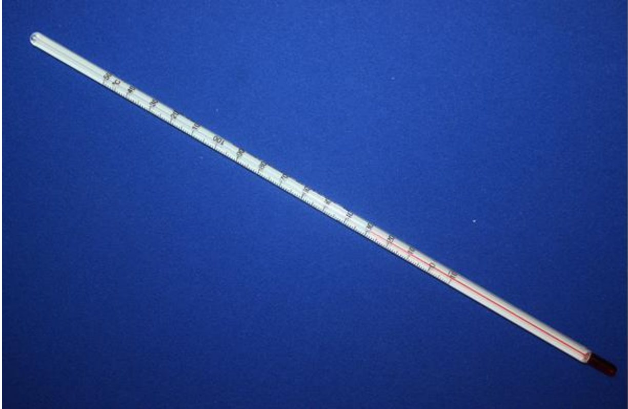
Figure 3-12: Red-alcohol filled thermometer used for the room's air temperature measurement
