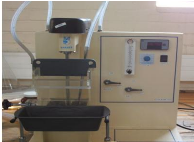
Figure 24: A photograph of the batch flotation cell
