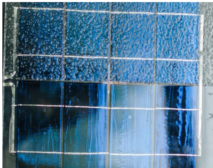
Figure 2.2: Solar roadway covered with a layer of translucent, tempered glass with a special non-adhesive coating
