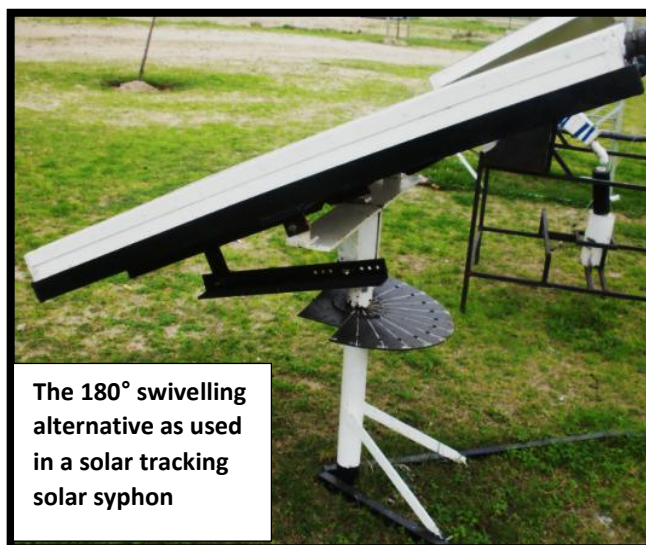
Figure 4.6: Possible alternatives to help achieve 0° and 180° azimuths with same installation: (Designs and photos by Kanyarusoke)
