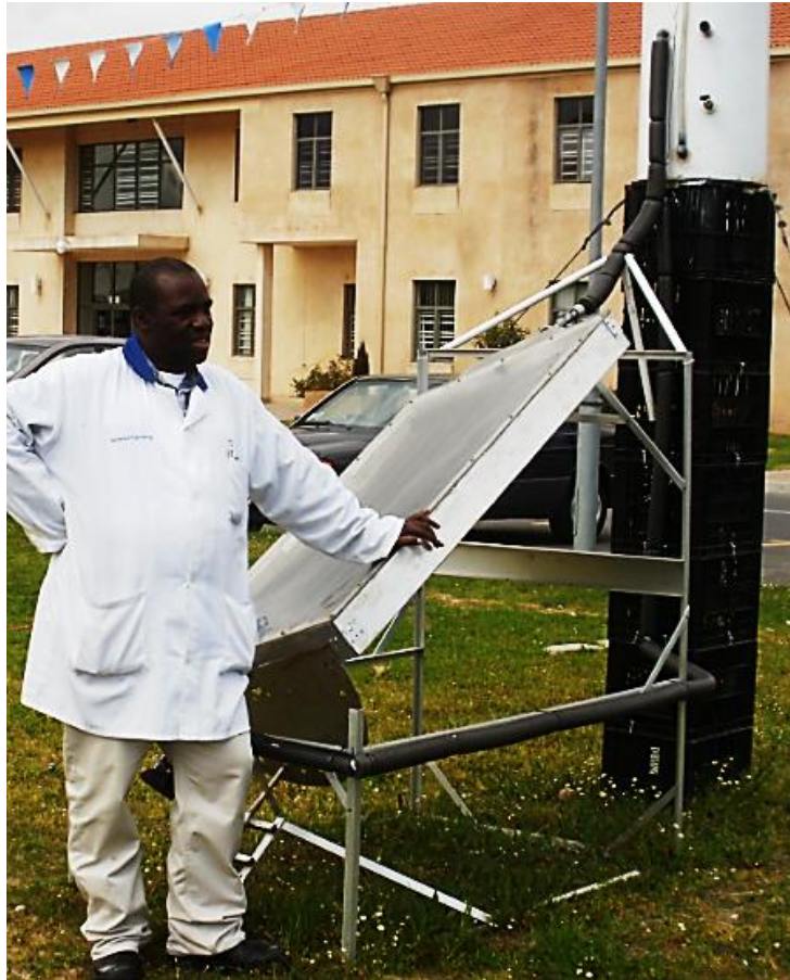
Figure 6.4: The Researcher and the inclined axis solar tracking solar syphon
