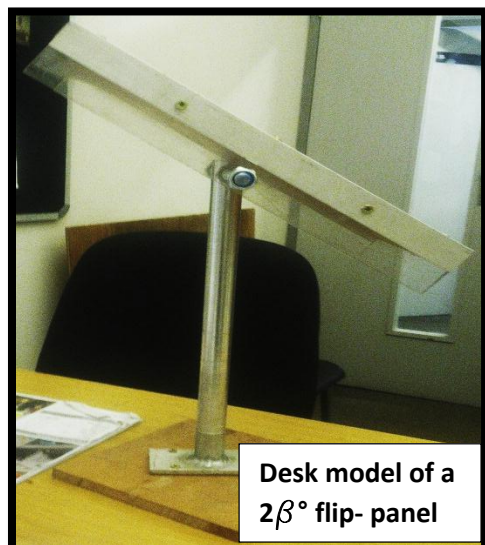
Figure 4.6: Possible alternatives to help achieve 0° and 180° azimuths with same installation: (Designs and photos by Kanyarusoke)
