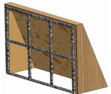
Figure A1.2: The back cover side with double sides self-adhesive net
