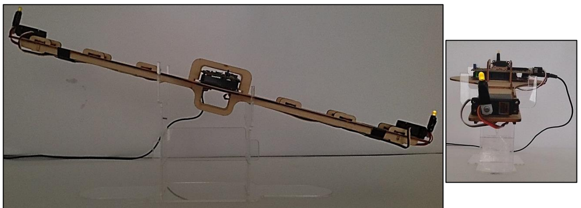
Figure 5.15: Physical model behaviour under ±15° roll and 0° pitch destabilisation
