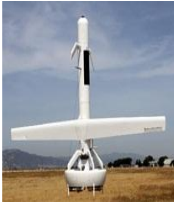
Figure 1.6: SiCX 300V Tail-siting UAVs (Guided System Technologies Inc, 2009)
