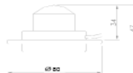
FIGURE 5. Dimensions of SP-LITE with Leveling Device
