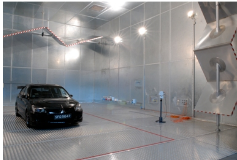
Figure 2.4: EMERL reverberation chamber for susceptibility measurements (From EMERL, 2007)
