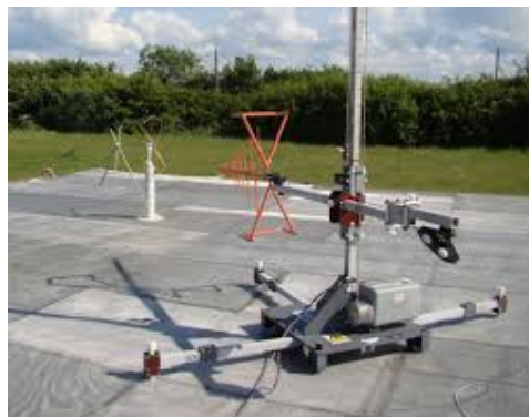
Figure 2.1: Open Area Test Site for antenna calibration testing as per CISPR 16-1-4 and CISPR 16-1-5 using a welded steel ground plane (From ETS-Lindgen)
