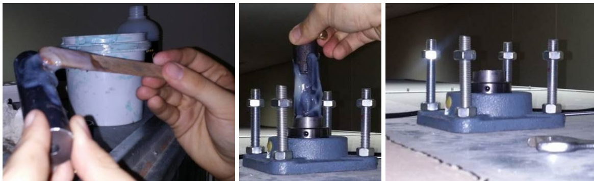
Figure 5.11: A solid cylindrical metal is glued to the stirrer shaft through the bearings; the stepper shaft is inserted at its other extremity
