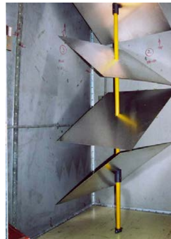
Figure 5.1: Different types of stirrers : (i) Z-fold stirrers, (ii) triangular-base stirrer with perpendicularly mounted paddles, (iii) Rot-Z stirrer, a fan-style stirrer used in the RC of the Defence Science and Technology Organisation, Australia, and (iv) NPL rectangular stirrer
