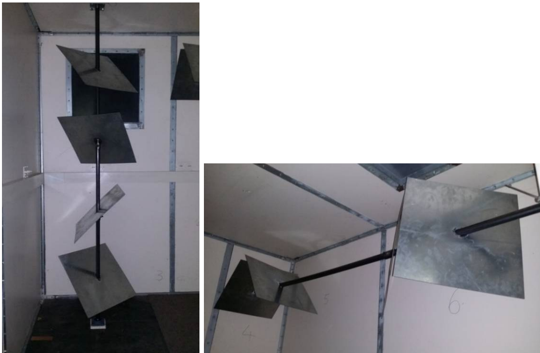
Figure 5.3: Vertical and horizontal mechanical stirrers placed in the RC
