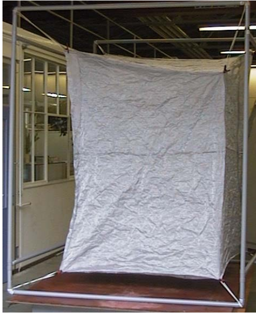
Figure 2.6: Vibrating Intrinsic Reverberation Chamber (From Leferink, 2000)
