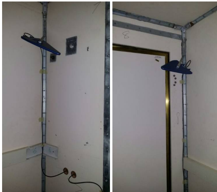
Figure 6.3: Transmitting and receiving antennas inside the reverberation chamber
