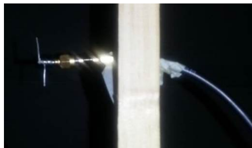
Figure 7.14: Short dipole antenna used instead of E-field probe
