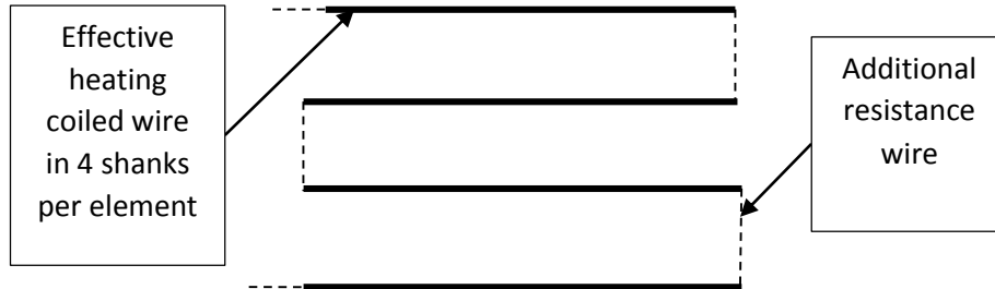
Figure 3.4: Schematic diagram of heating elements of the furnace
