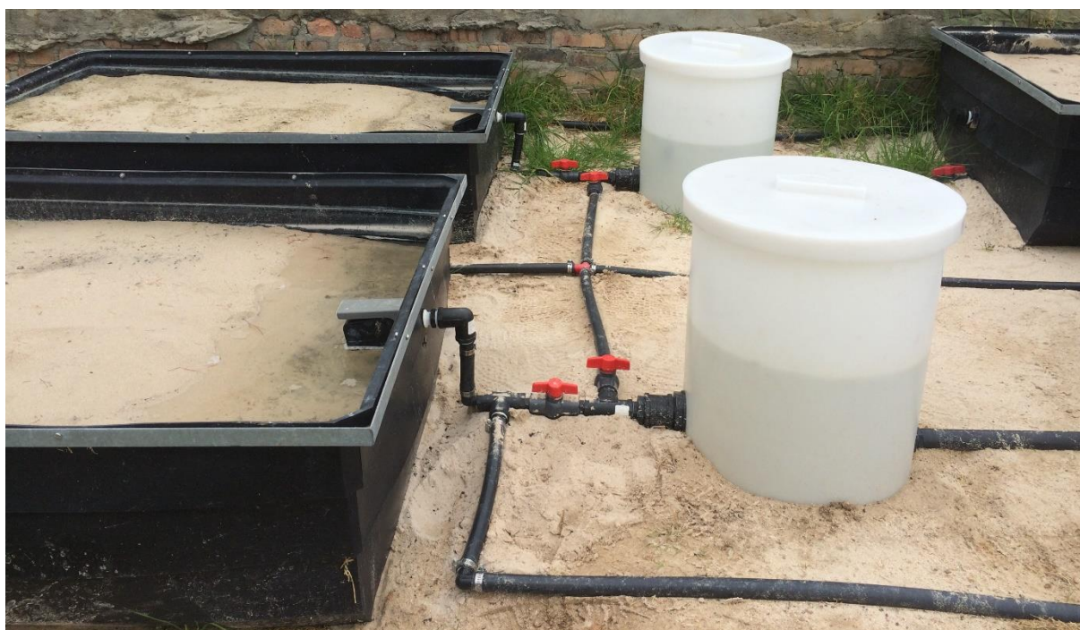
Figure 3.5 A picture showing the set-up of the pipes and control valves that allow the system to be operated in series or in parallel
