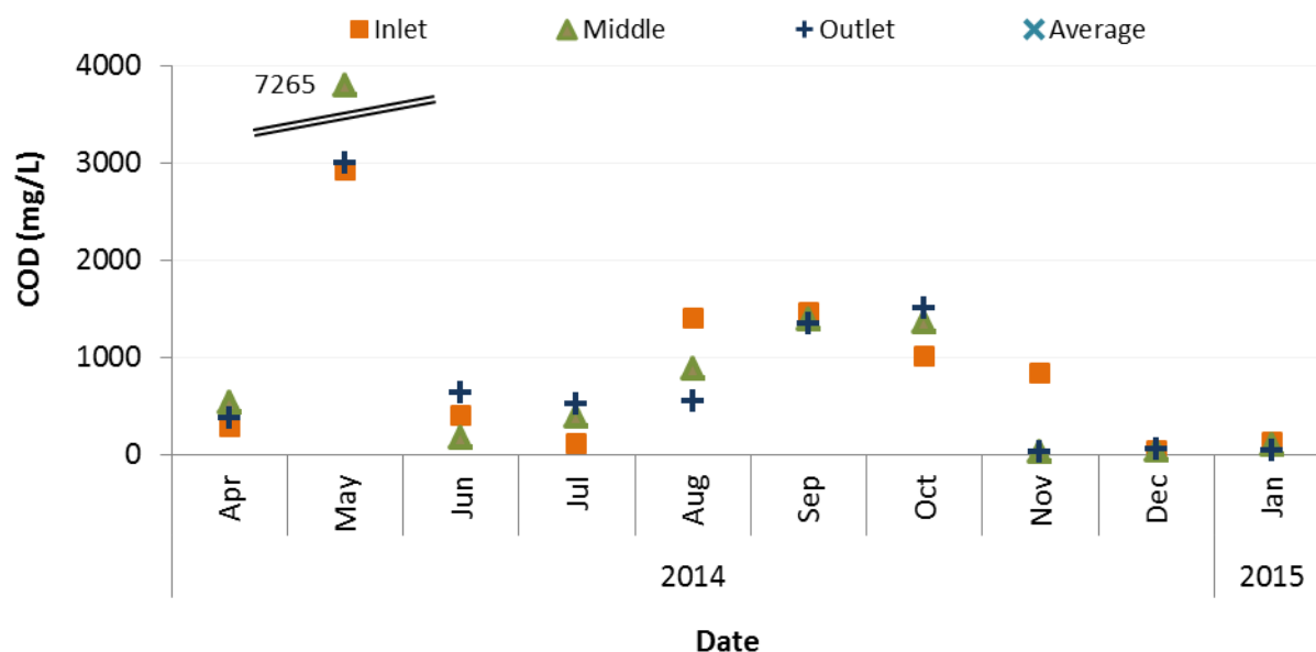
Figure 4.2 Chemical oxygen demand concentrations measured in samples from the existing settling basin at the inlet, middle and outlet sampling points before commissioning of the BSF system, Apr 2014 – Jan 2015
