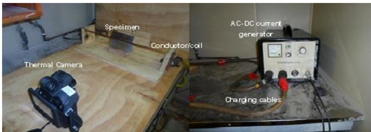
**Figure 3-33. Typical experimental setup for Induction Thermography**
