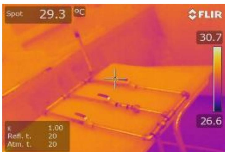
**Figure 3-5. Thermal image of model's pipe network before experiment**
