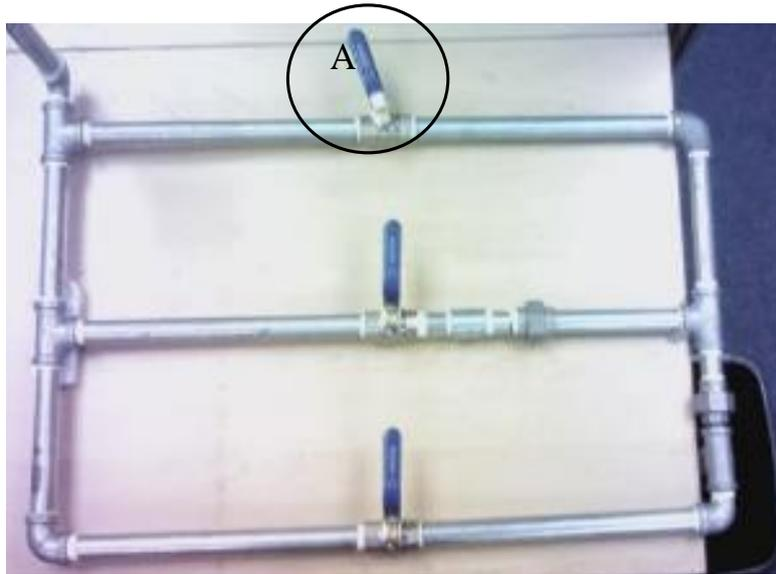
**Figure 3-4. Fluid handling model with valve A cracked open**
