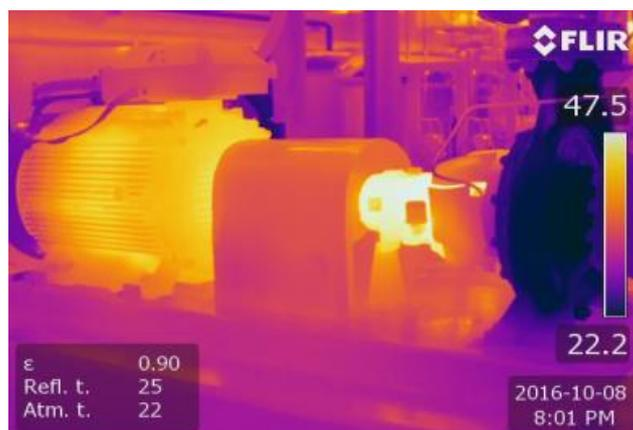
**Figure 2-3. Thermal profile of the in-service pump shown in figure 2.2**
