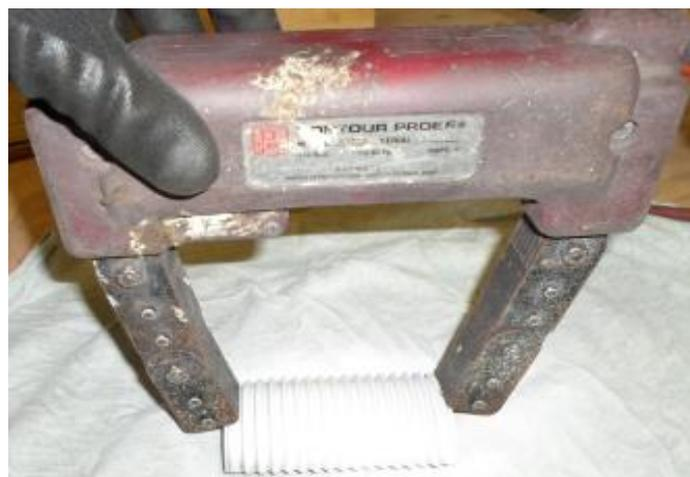
**Figure 3-37. Experimental set-up of MPI with the turbine's stud**
