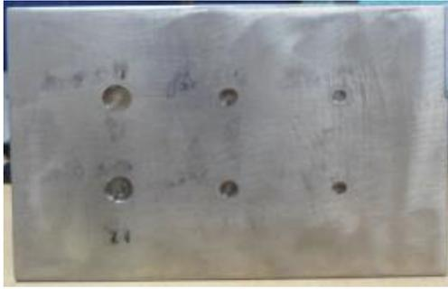
**Figure 3-18. Rear view of the specimen with machined defects**
