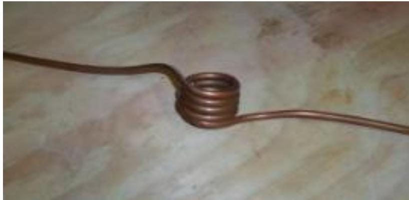
**Figure 3-32. Coil used for CV-joint inspection**
