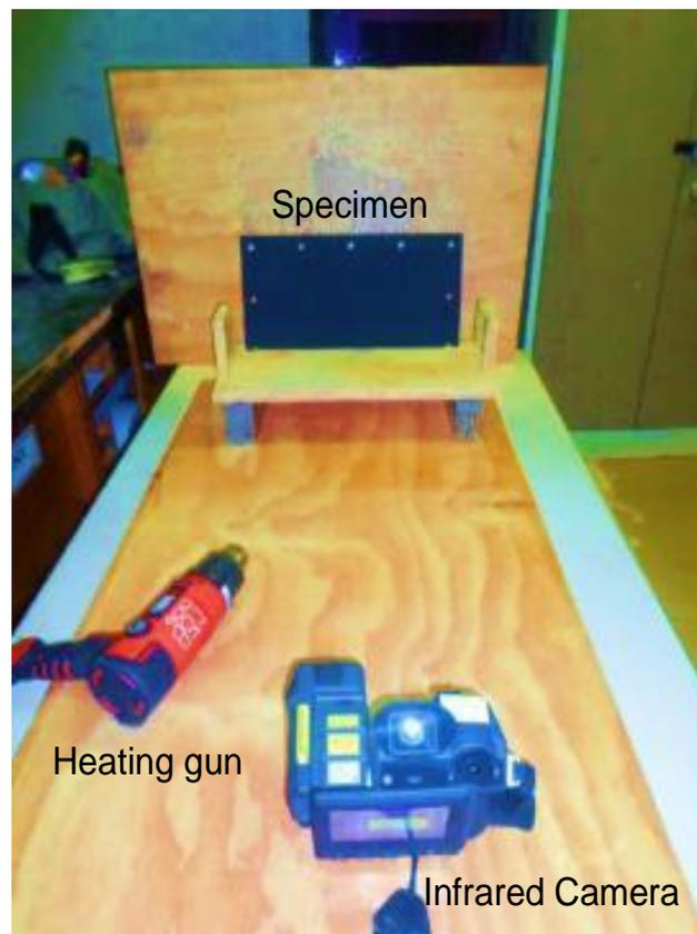
**Figure 3-17. Illustration of equipment used during pulse thermography**
