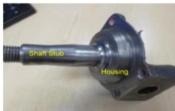
**Figure 3-31. CV-joint**
