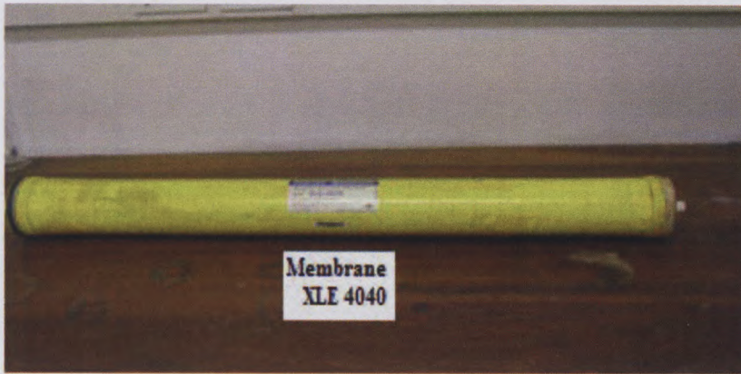
Figure 5-1: Photograph of the membrane to be autopsied
