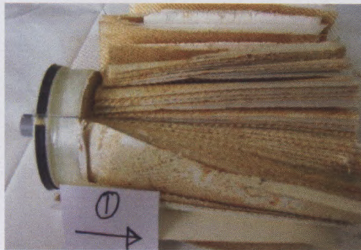
Figure 5-3: A photograph of the autopsied part of the membrane
