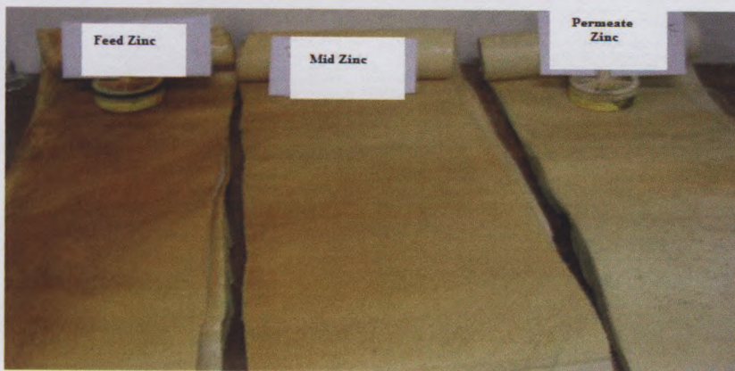
Figure 5-5: Photograph of membrane (treated with Zn^{2+} ions) cut into three parts
