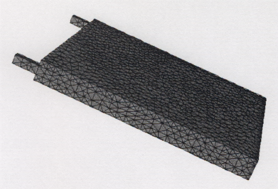
Figure Appendix B.9: 3-D meshing model for capacitive accelerometer
