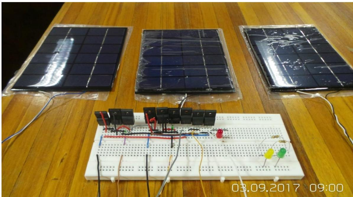
**Figure 8.11:** Experimental Set up for measurement of the produced output
