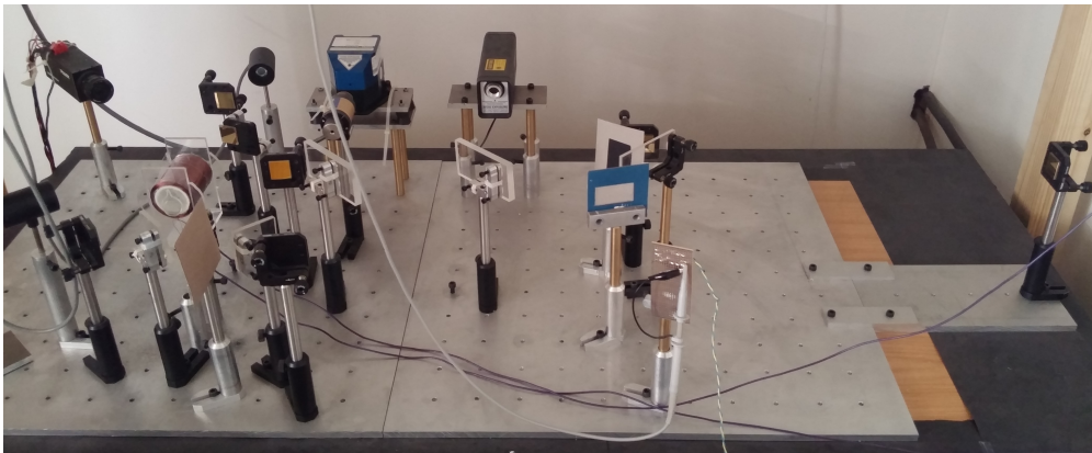
Figure 3.2: Arrangement 1 of our saturated absorption spectroscopy (SAS) setup in the laboratory. Two aluminium base plates are seen: the left plate is the SAS setup and the right is the Michelson interferometer. A helium-neon laser is included in the setup to perform beam alignment.
