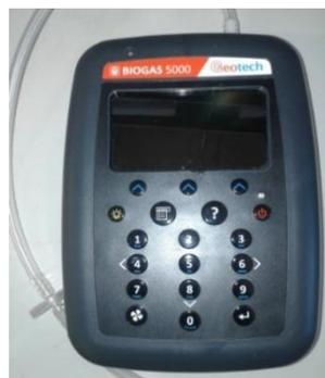
**Figure 13: Biogas analyser used to determine the composition of the biogas**
