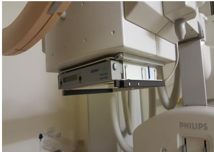
Figure 2.1: Retrofitted Dose Area product (DAP) meter with reading display on the Philips unit at the research site
