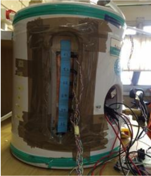
Figure 6.3 Temperature sensors on side of geyser for temperature monitoring
