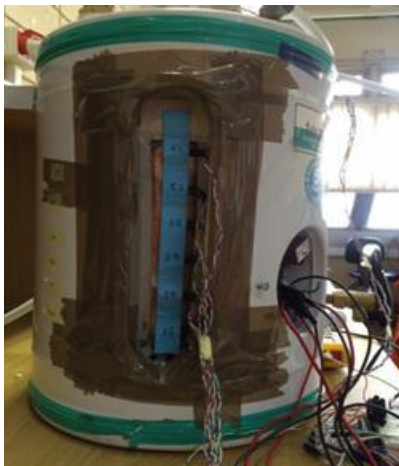
Figure 4.11 Six LM35 temperature sensors along the side
