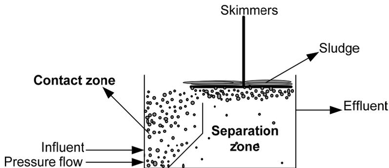
**Figure 3.1: Schematic illustration of the contact and separation zones of a dissolved air flotation system (Behin & Bahram, 2012; Edzwald 2010)**
