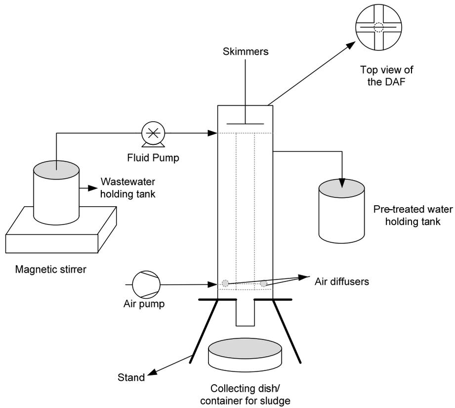
**Figure 4.2:** Schematic illustration of the DAF bench scale set up.
