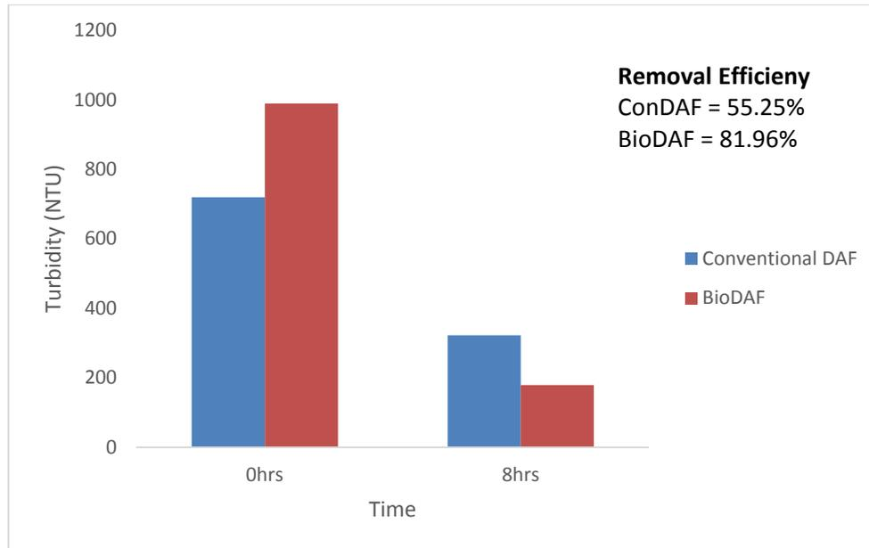
**Figure 5.7:** Graphical illustration of turbidity reduction (ConDAF vs BioDAF)
