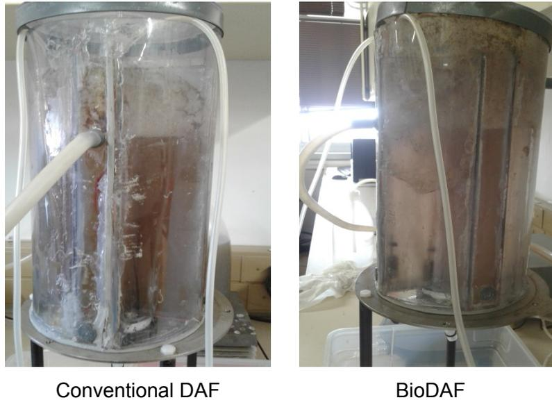
**Fig C1: Photographic representation of Con DAF vs BioDAF during a pre-treatment process**
