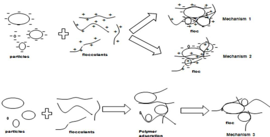
**Figure 2.3:** Representation of flocculation mechanism (1) charge neutralization, (2) electrostatic patch and (3) polymer adsorption and bridging (Dao *et al.*, 2016).
