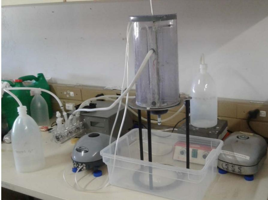
**Figure 4.1:** Photographic illustration of the DAF bench scale set up.
