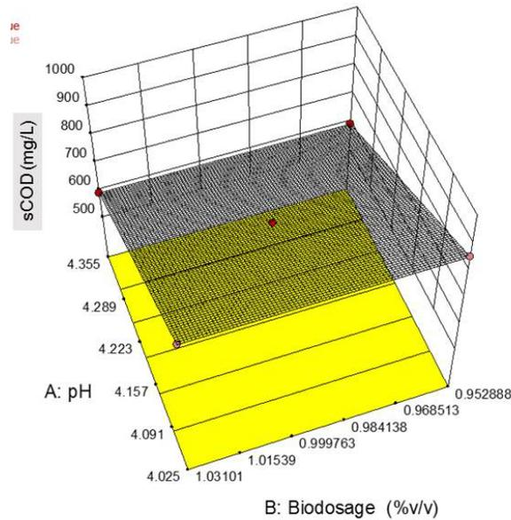
**Figure 5.10:** 3-D surface plot showing the interaction of bioflocculant dosage and pH on sCOD removal.
