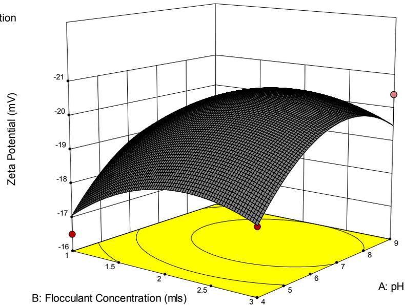
**Figure 5.4:** 3-D surface plot showing the interaction pH and bioflocculant dosage on zeta potential
