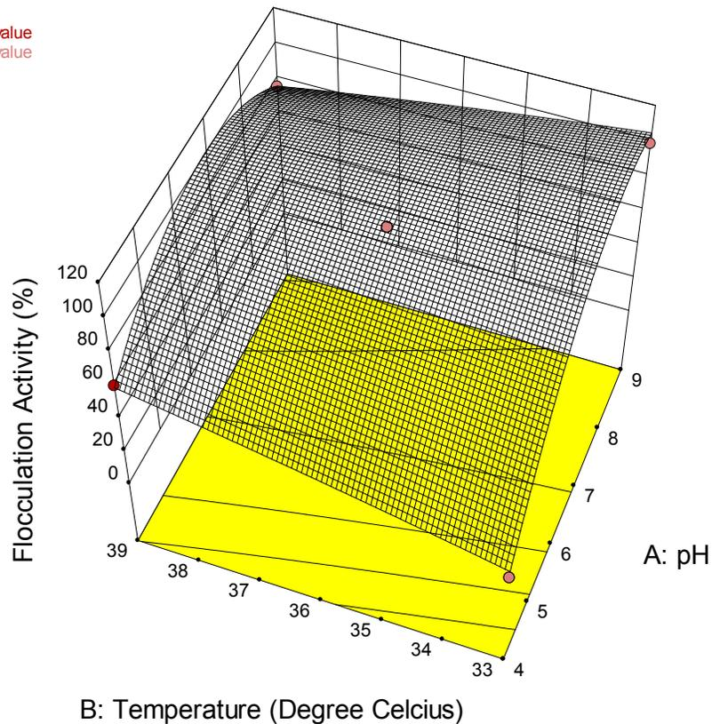
**Figure 5.2:** 3-D surface plot showing the interaction of temperature and pH on flocculation activity
