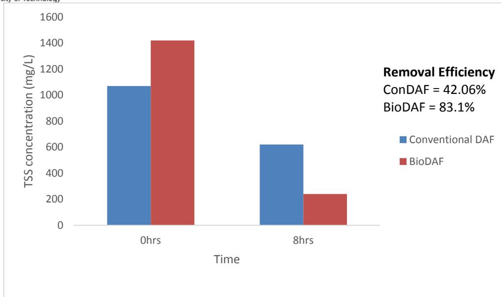
**Figure 5.6:** Graphical representation of TSS concentration reduction (ConDAF vs BioDAF)
