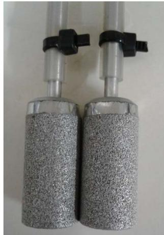
**Figure 4.3:** Specifically designed air diffusers used in the DAF system.
