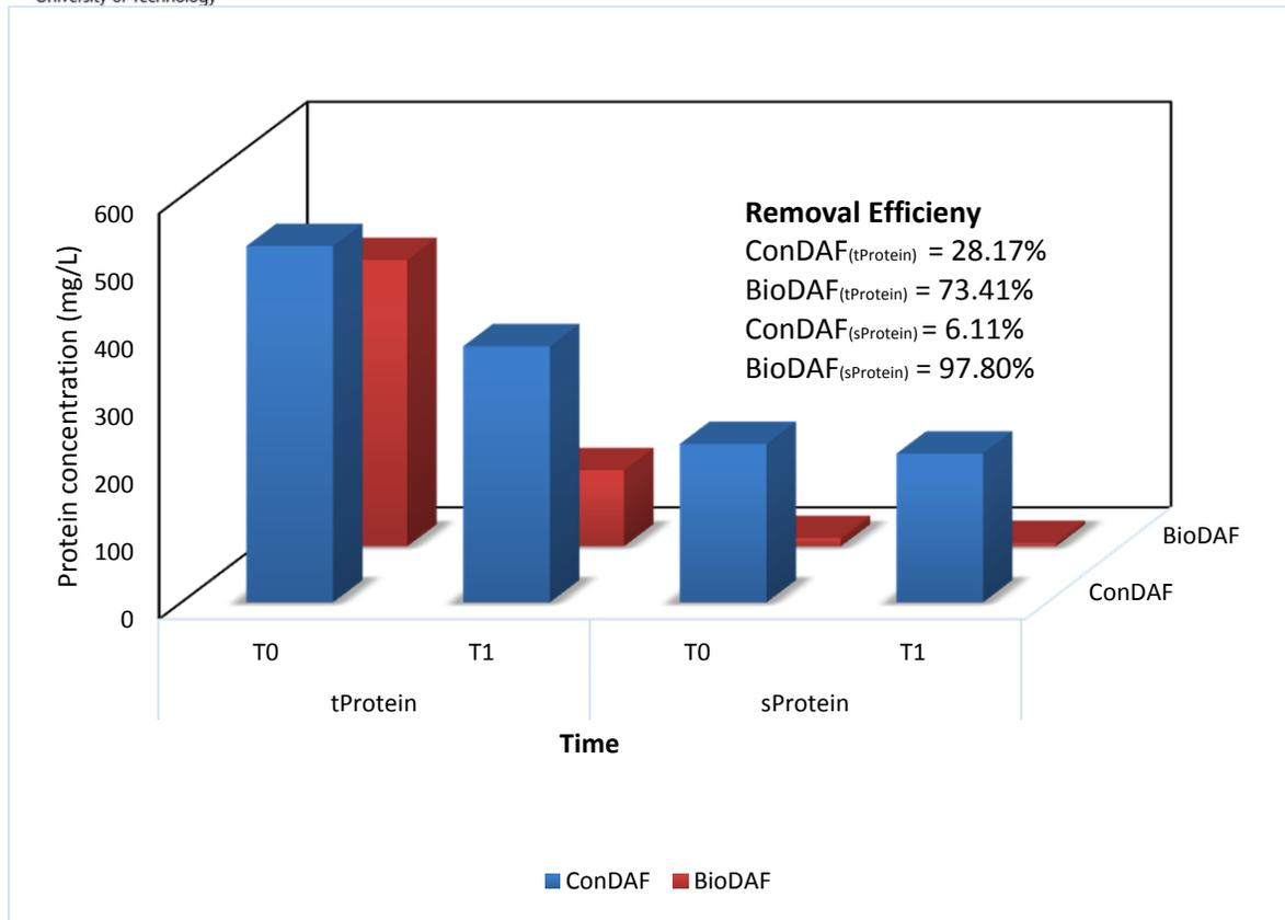
**Figure 5.9:** A representation of protein concentration reduction (ConDAF vs BioDAF)
