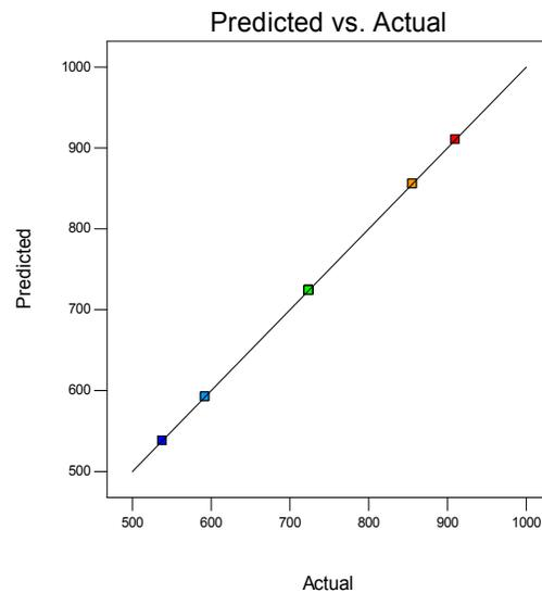
**Figure 5.11:** Graphical representation of predicted vs actual sCOD removal efficiency
