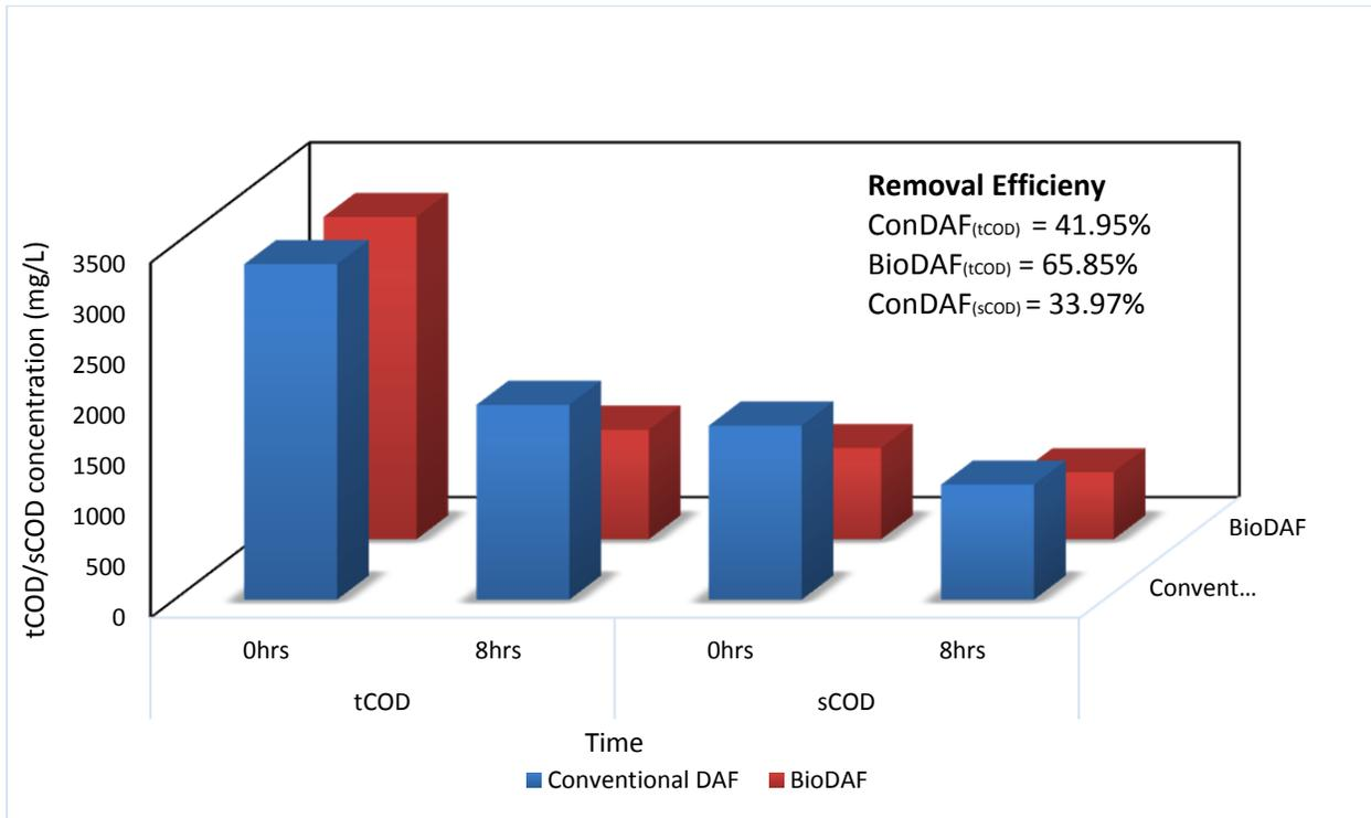
**Figure 5.8:** Graphical profile of tCOD and sCOD reduction (ConDAF vs BioDAF))
