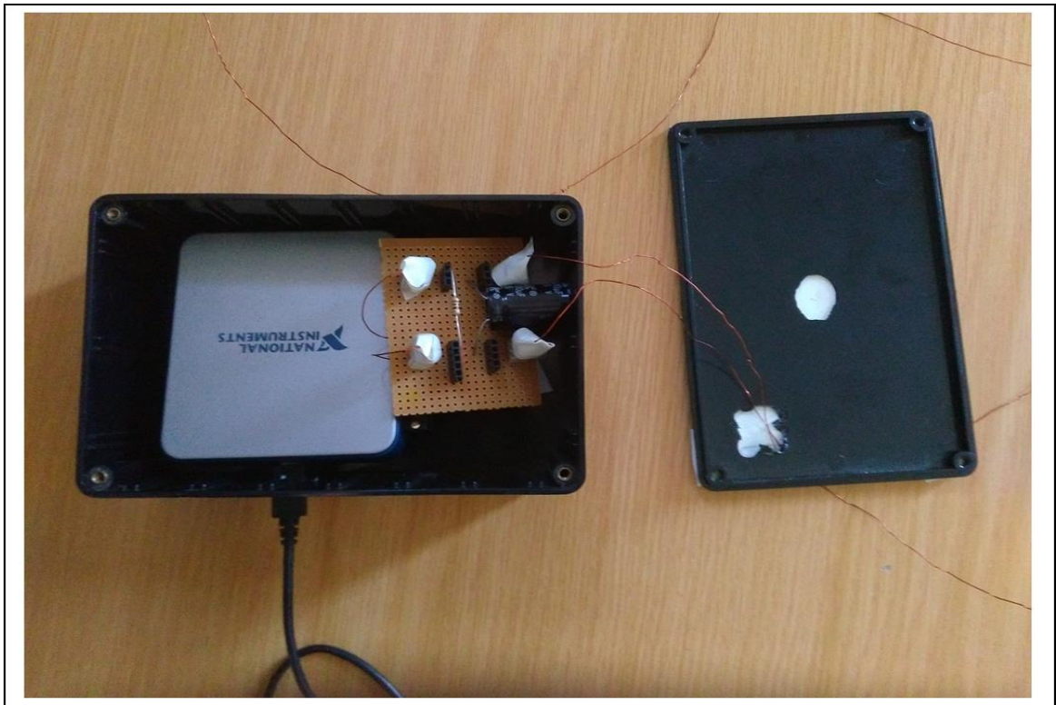
Figure D.3: Photos of the measurement circuit and Labview NI-DAQ device inside a plastic case.
