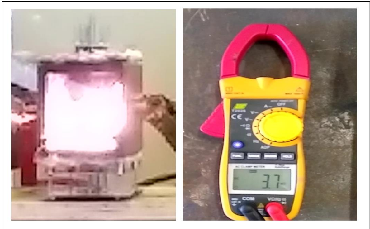
Figure E.6: Photos illustrating the rectangular duct with plasma and the measured terminal voltage (3.7 mV) from a multimeter.
