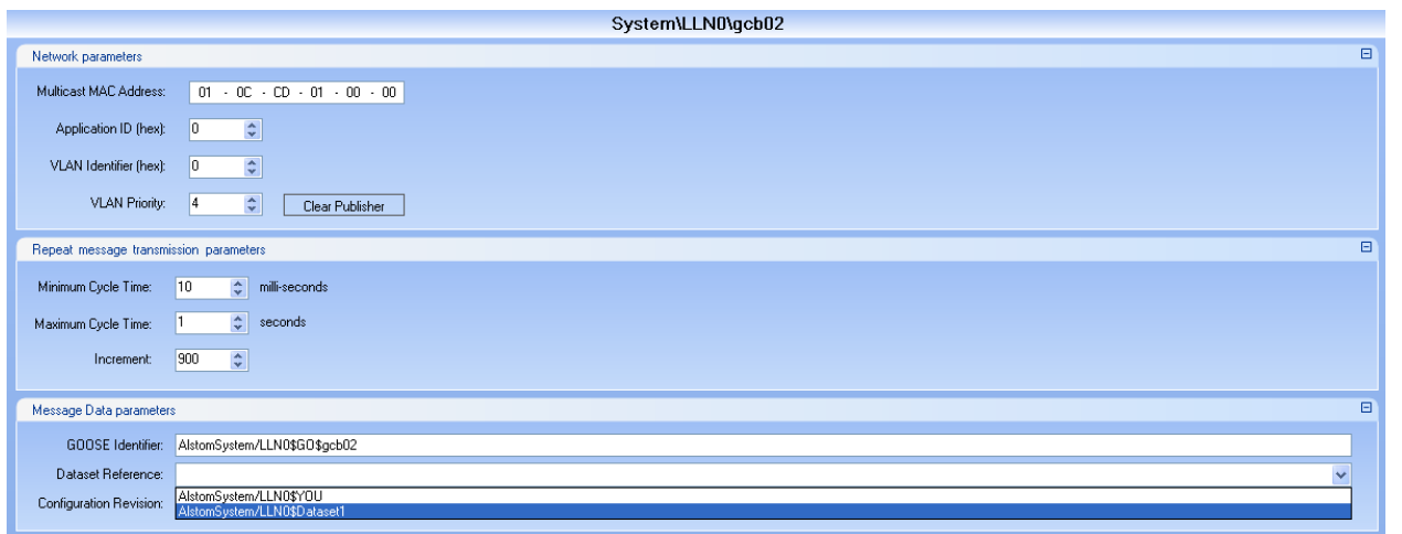
Figure 6.107: GOOSE control block
