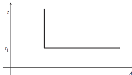
Figure 5.4: Definite Time Relay Characteristics Curve
