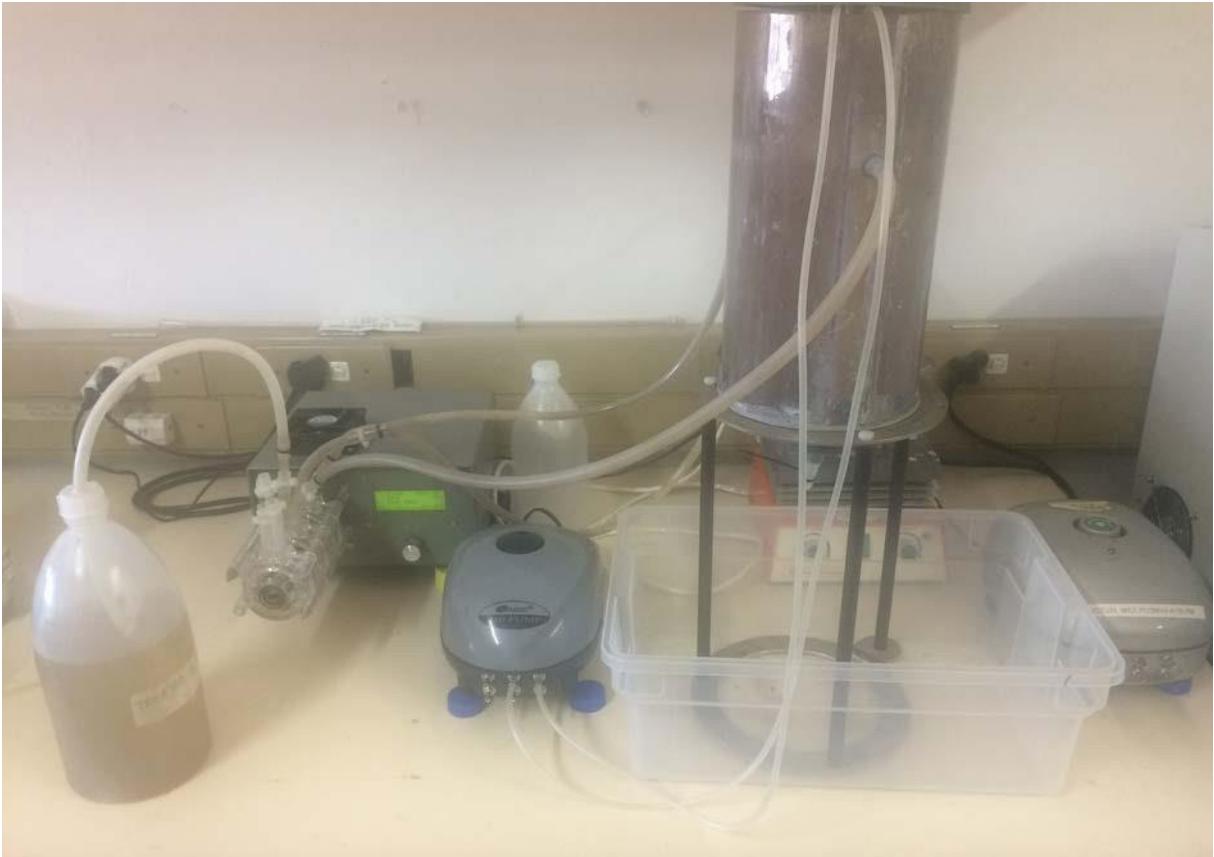
Figure 3-1: Dissolved air flotation (DAF) used in this study.
