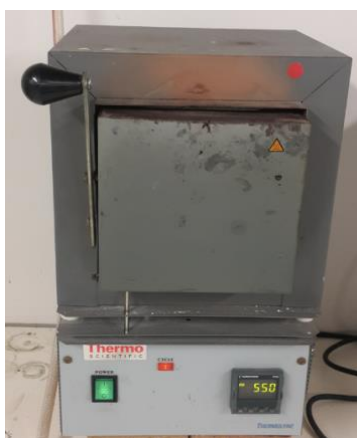
Figure 3. 2: Experimental set up of the fusion process of the as-received fly ash with NaOH set at 550 °C for 1 hour 30 minutes (Refer to images in Figure 4.2 micrographs)
