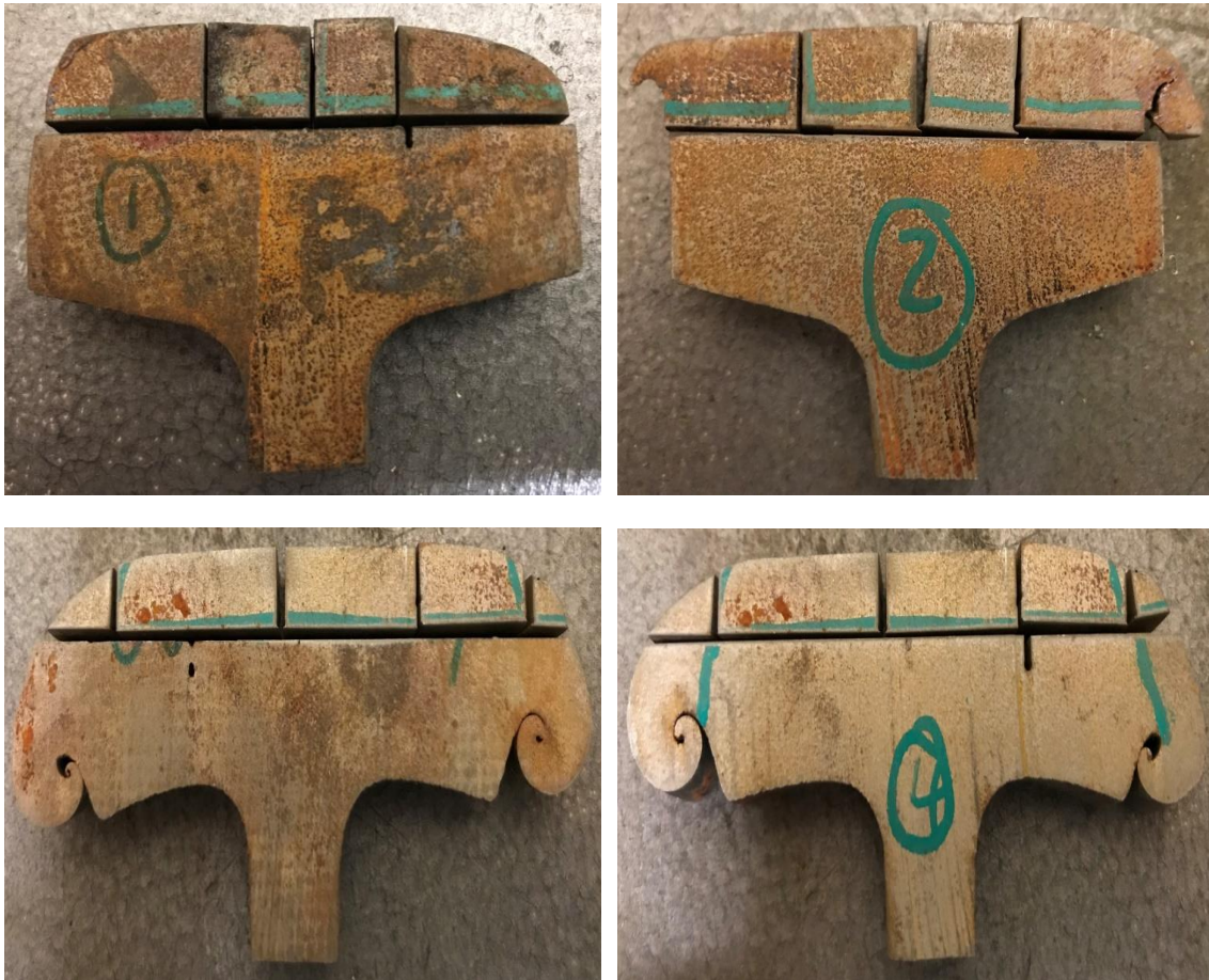
Figure 3.2: Steel rail sample cut into four 10mm pieces
