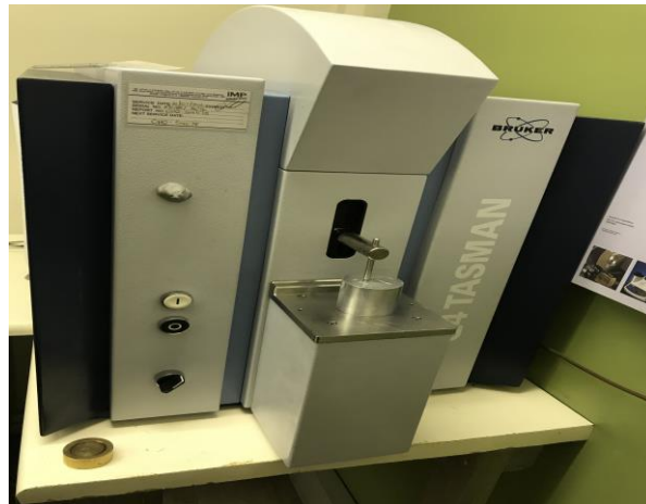
Figure 3.5: Q4 Tasman scanning electron microscope (SEM) coupled with electron dispersion X-ray spectroscopy (EDX)
