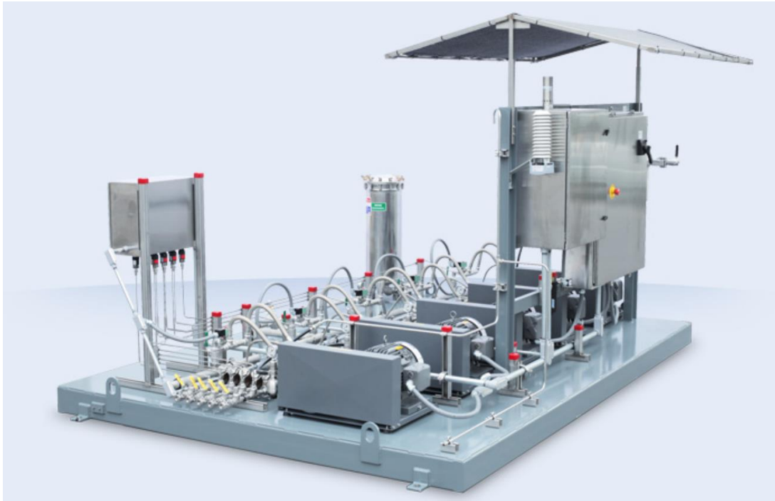
Figure 5.1: MEE fog high pressure fogging system (Envitech 2014)
