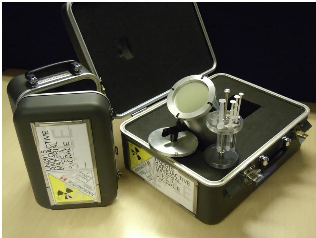
Figure 4: Type A packaging for transporting radioactive waste (Sorenson, 2015)
