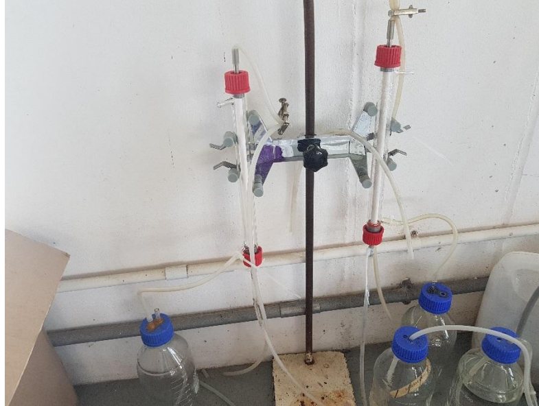
Figure 3-8: UF membrane system set-up
