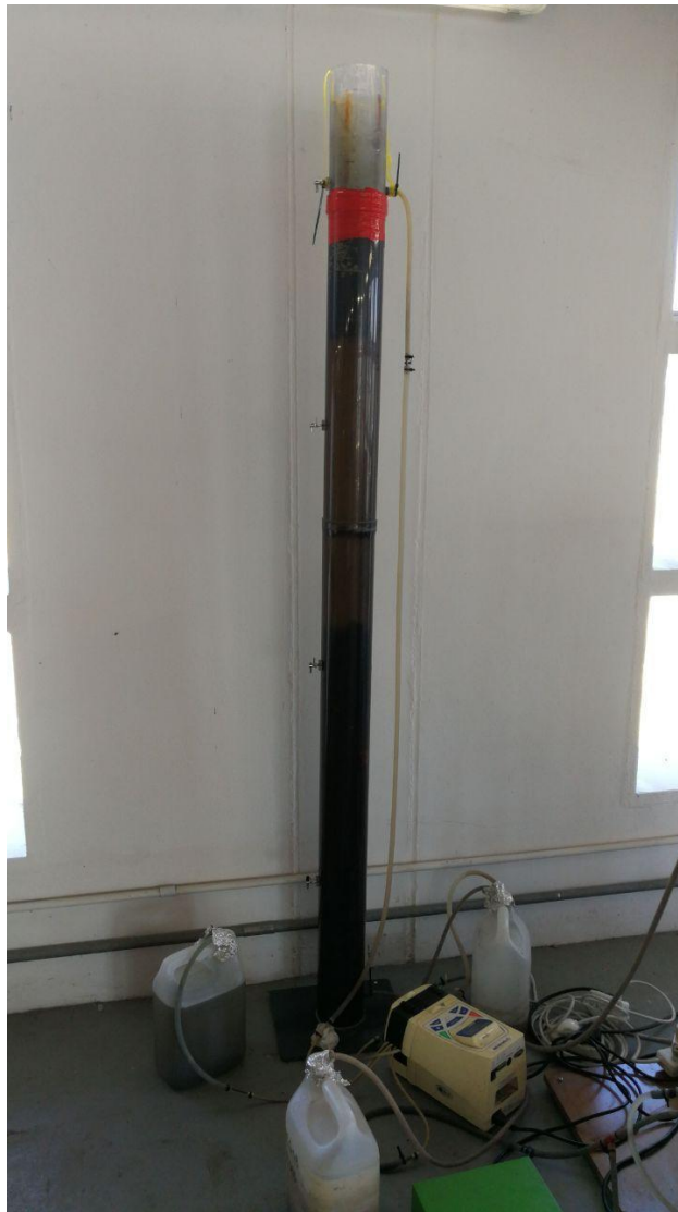
Figure 3-5: Single stage nitrification and denitrification Set-up
