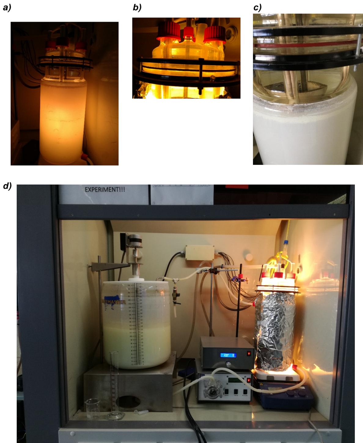
Figure 3.10: Photoreactor and the system, a) photoreactor without the reflective sheet, b) reactor clamping system also illustrating the lamp housing system, c) illustrates the internal reflective disc and d) the complete system illustrating the photoreactor in operation with the external reflective aluminum sheet
