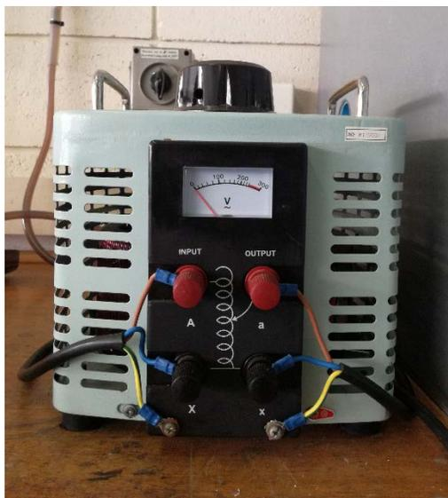
Figure 3.15: 5kVA transformer
