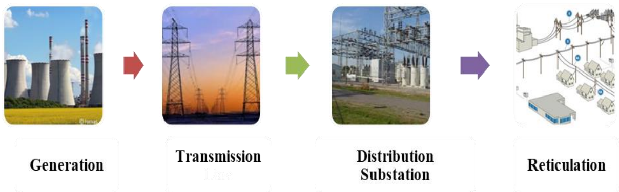
Figure 4.1: Traditional power grid, characterized by generation, transmission, distribution and reticulation of electricity to end-use consumers. Image Source (EPRI, 2014)
