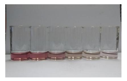
Figure 4.21: Visible degradation of the mixed dyes batch over time
