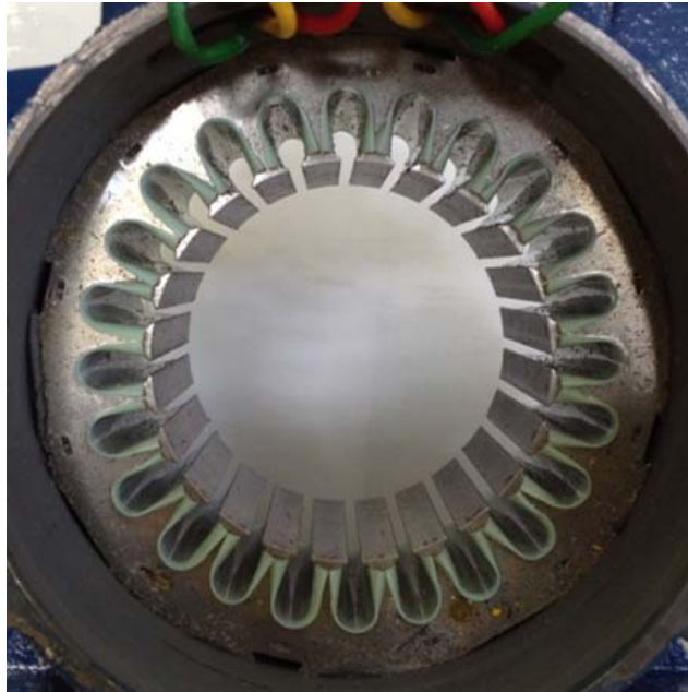
Figure 4-5: A clean stator after removal of the windings
