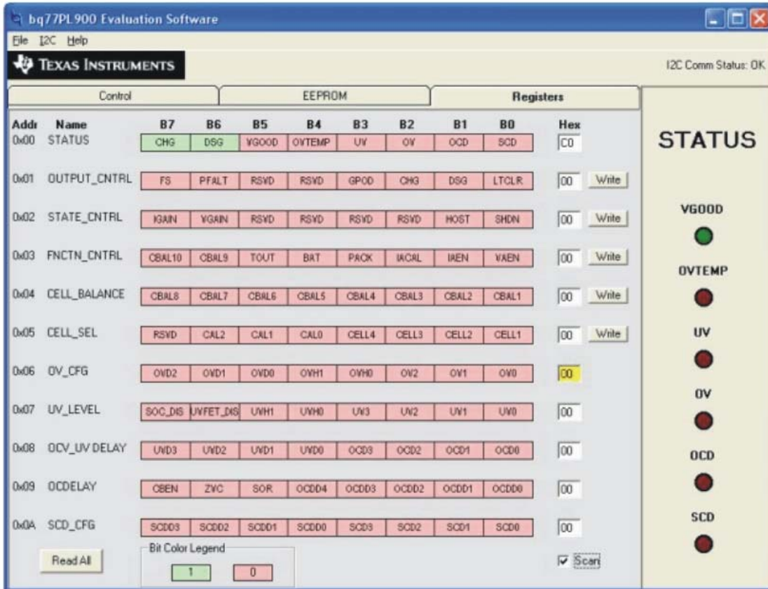
Figure 5-11: Interface of addressable registers (Texas instruments, 2018).
