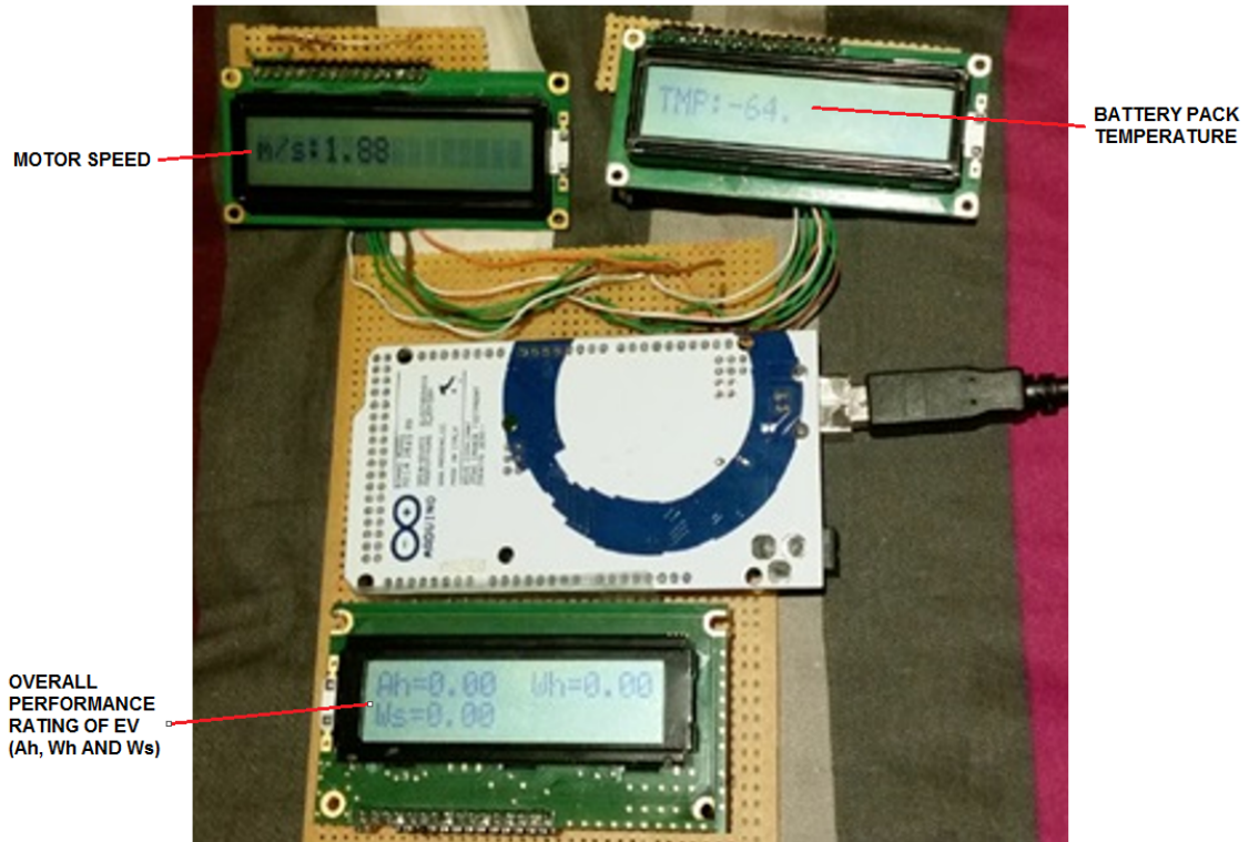
Figure 6-11: LCD configuration adjusted to fit into the EV dashboard
