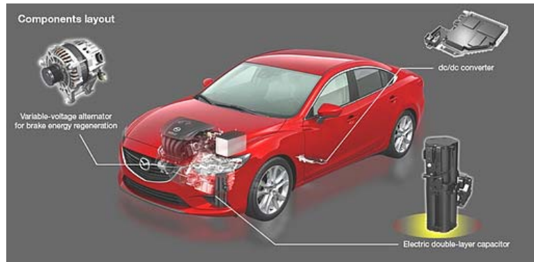
Figure 2-5: A super capacitor electric vehicle (SAE International, 2016)
