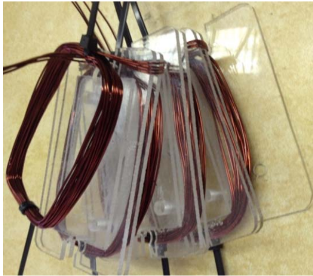
Figure 4-10: Completed Perspex jig with completed stator winding for one phase
