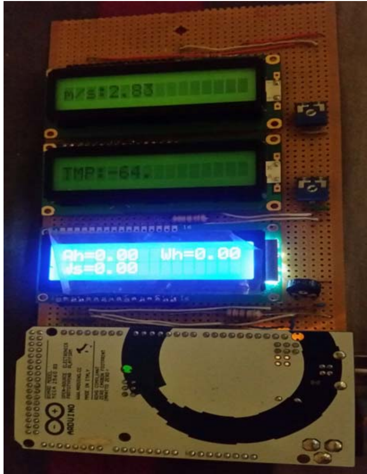
Figure 6-10: Testing the LCD functionality with the microcontroller
