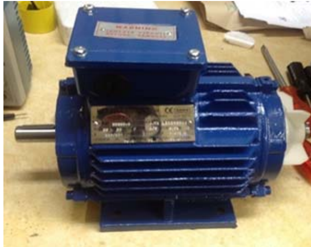
Figure 4-1: The Motorelli three-phase, squirrel cage induction motor
