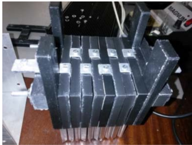
Figure 5-3: The assembly of one stack of ten cells
