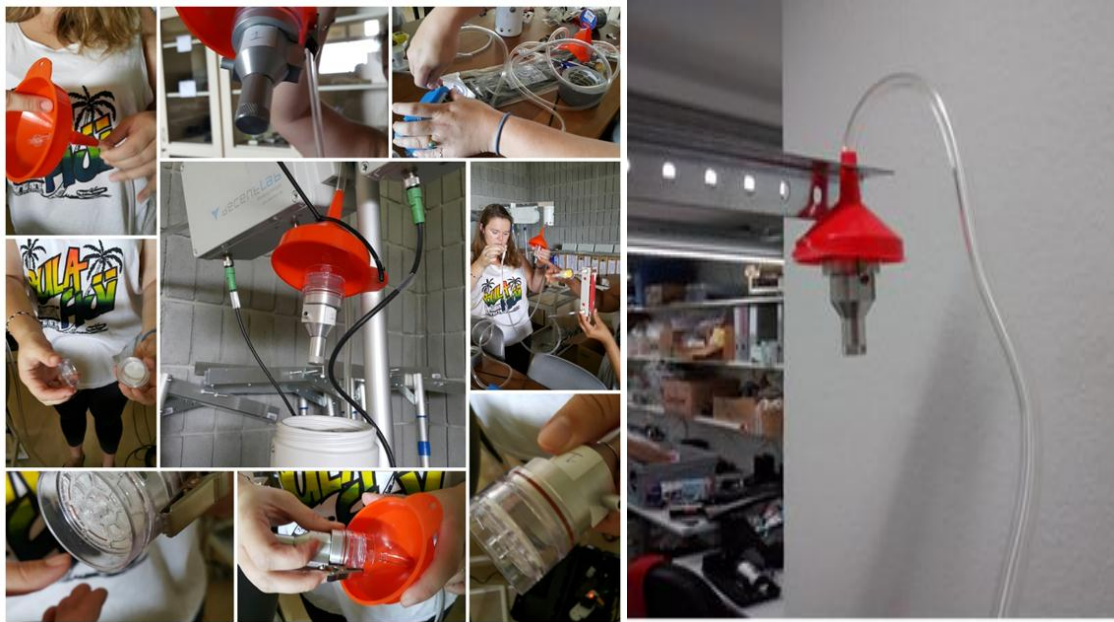
Figure 3.5: Tubing attached to centrifugal cyclone used for particulate matter
