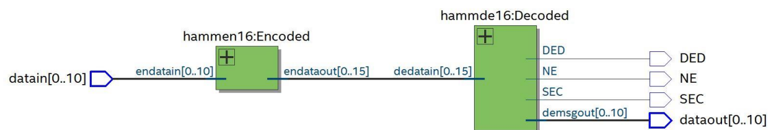
Figure 4-10: I/O overview of VHDL code (hamming_11_16_main.vhd)
