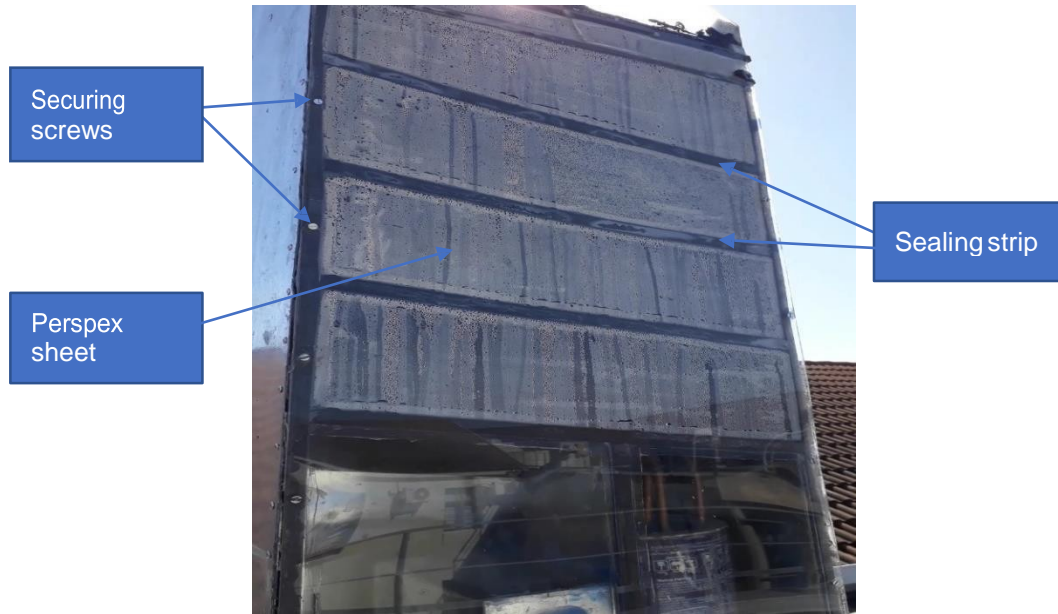
Figure 3.17: Front view of the multistage covered with perspex sheet
