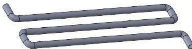
Figure 3.13: Stage one zig-zagged seawater tube
