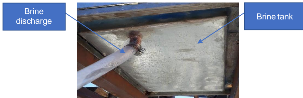
Figure 3.27: Brine tank located on the underside of the system
