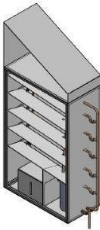
Figure 3.33: 3D view of the multistage solar still desalination system
