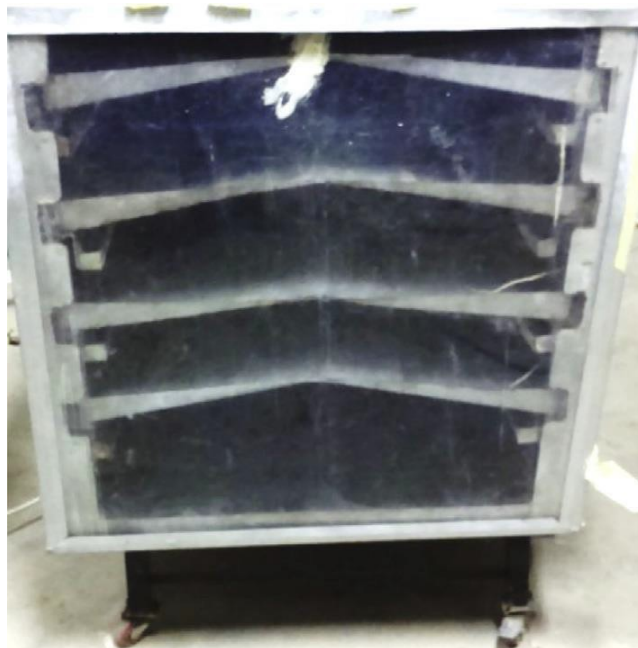
Figure 2.5: A-shaped stage trays (Abdessemed et al., 2018)
