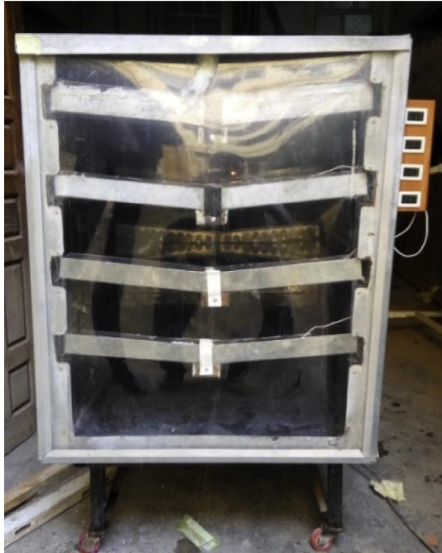
Figure 2.4: V-shaped stage trays (Abdessemed et al., 2018)
