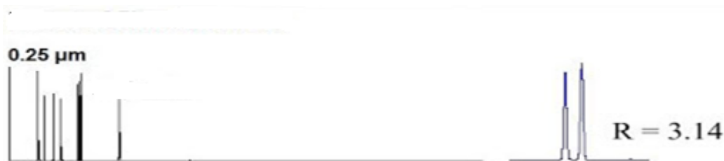
Figure 2.5 Chromatogram of 0.25 \mu\text{m} film thickness shows a decrease in retention run time
