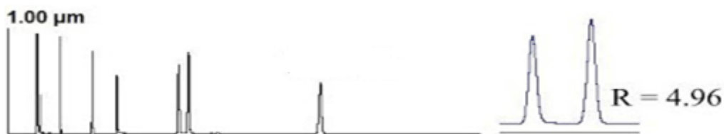
Figure 2.4 Chromatogram of 1.00 \mu\text{m} film thickness shows an increase in retention run time
