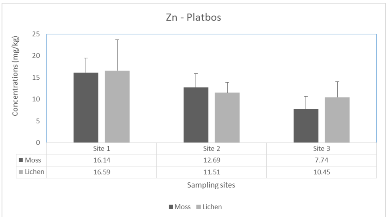
Figure 3.10: The mean Zn concentrations (mg/kg) ( \pm SD) in moss and lichen at sites 1, 2 and 3 of Platbos forest for the sampling occasion in May 2014. N=5.
