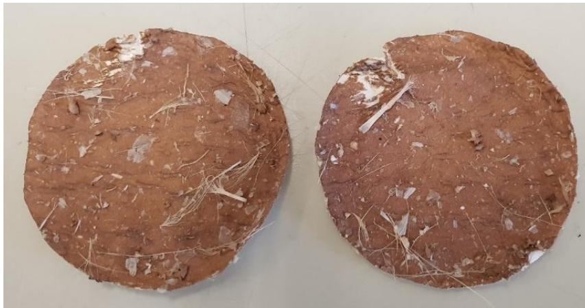
Figure 4.4: Image showing the residue of PWS on the 1.0 µm glass fibre filter after filtration.
