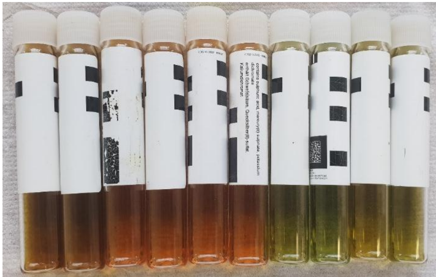
Figure 4.5: COD fractions (Total, filtered and flocculated filtered COD) in analysis test tubes
