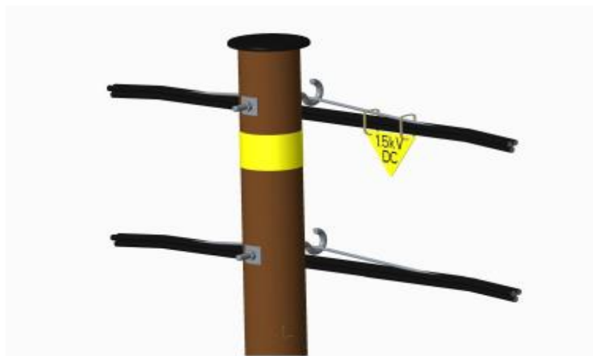
Figure 3. 28: Aerial bundled cable with notification stripe between lines connected to different voltage levels(Kaipia et al., 2017).
