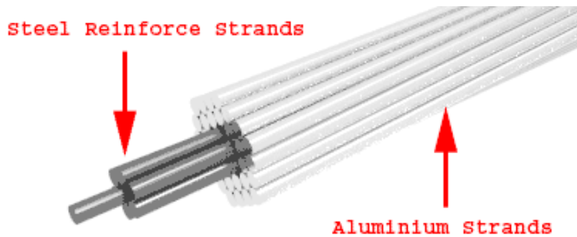
Figure 2.6: Aluminium conductor steel reinforced (electrical4u, 2017).
