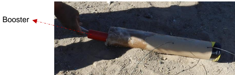
Figure 4. 13 Blasting pipe (40 mm diameter, 0.5 m long) with booster
