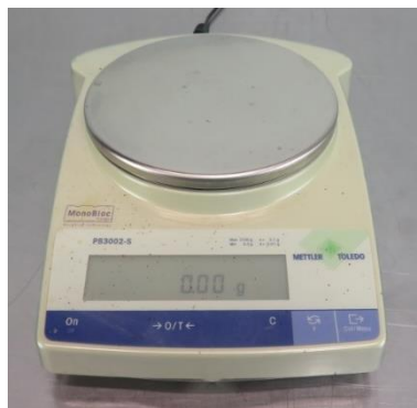
Figure 4. 3 Mettler Toledo PB300-S laboratory balance (error: \pm 0.003 g)
