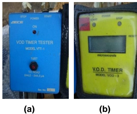
Figure 4. 11 (a) VOD time tester model VTT-1 (b) and VOD timer model VOD-3
