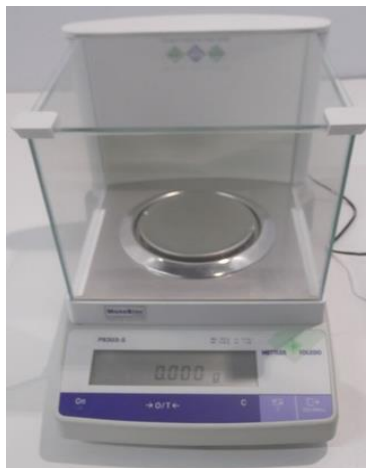
Figure 4. 1 Mettler Toledo PB303S-2T balance (error: \pm 0.0002 g)
