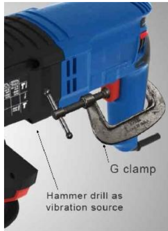
Figure 3.22 Control of vibrational frequency by pressing the speed button of the hammer drill, using a G clamp.
