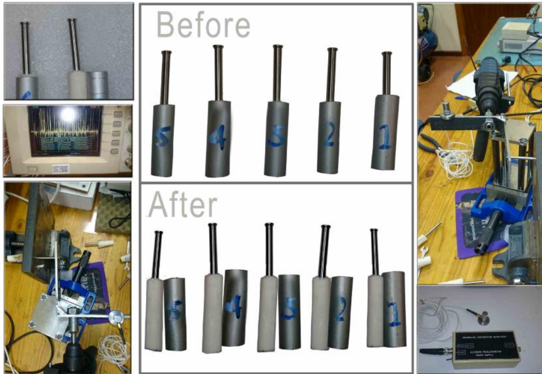
Figure 3.25: Using vibration at a frequency of 40 Hz and varying the distance between the pivot point and the implant’s head. Recording the time when positive result occurred.
