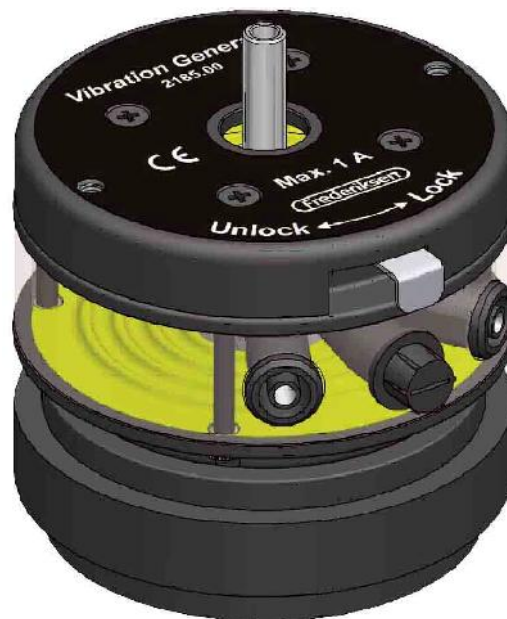
Figure 3.8: A Laboratory Vibrations Generator
