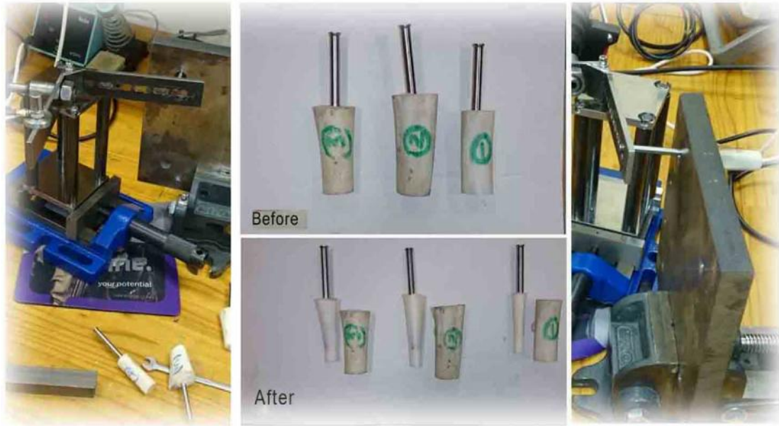
Figure 3.26: Positive results with animal bones encasing the cement and implant at optimum distance and frequency of vibration.
