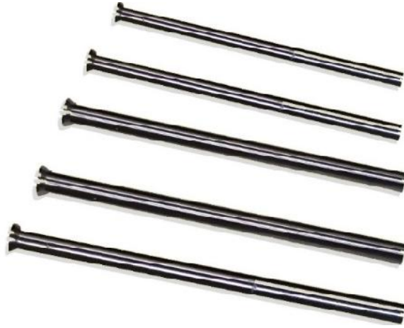
Figure 3.15 Metal rods used as 'implants' for small samples
