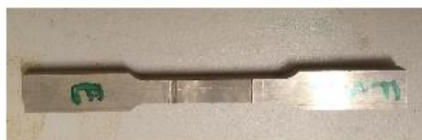
Figure 3.4.1: (b) Sample of a tensile test specimen.
