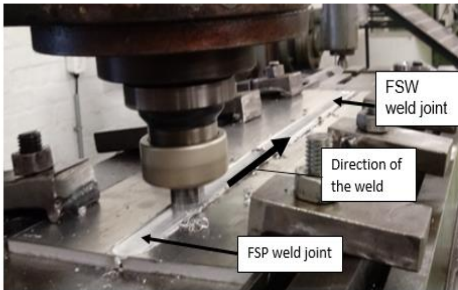
Figure 3.2.3: (a) FSP application on FSW welded joint.
