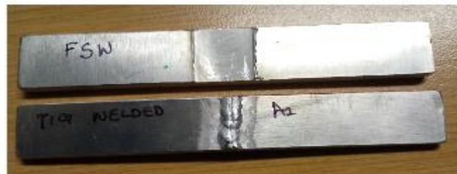
Figure 3.4.2: (b) Sample of a bending specimen.
