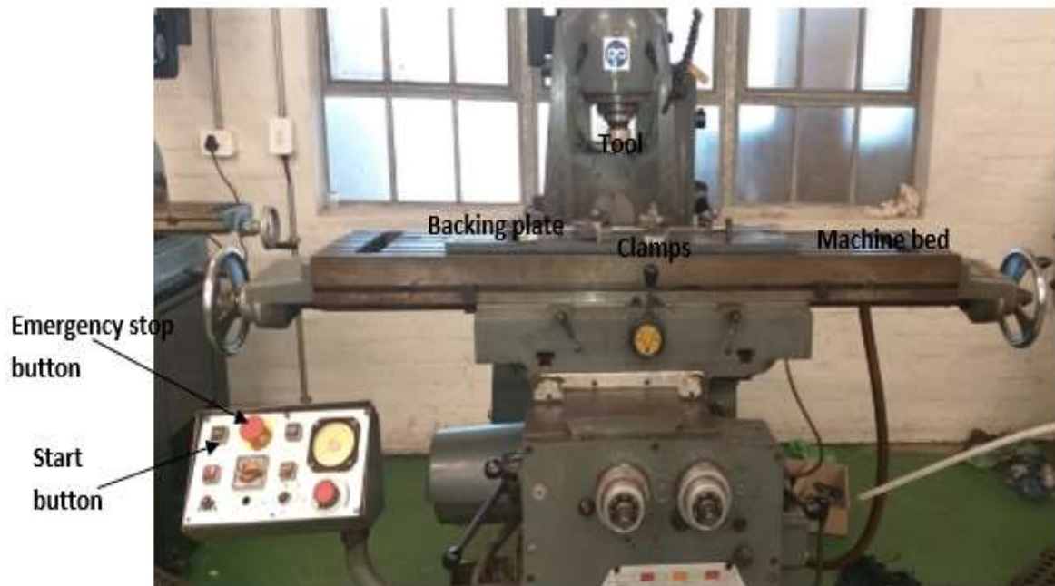
Figure 3.2: Semi-automated milling machine
