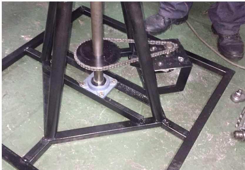
Figure 3-12: CSPVT solar tracker: chain and sprocket arrangement
