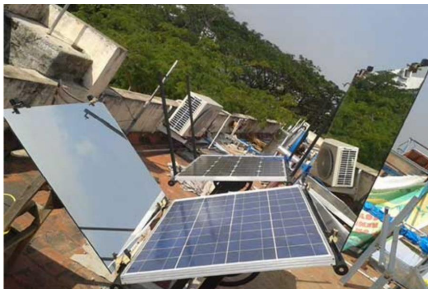
Figure 2-9: Prototype of a V-through solar collector created at Anna University, Chennai. Source: V-trough solar collector, (Nivas, n.d.)
