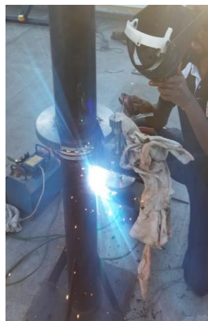
Figure 3.25: Welding gearbox to the stationary pillar
