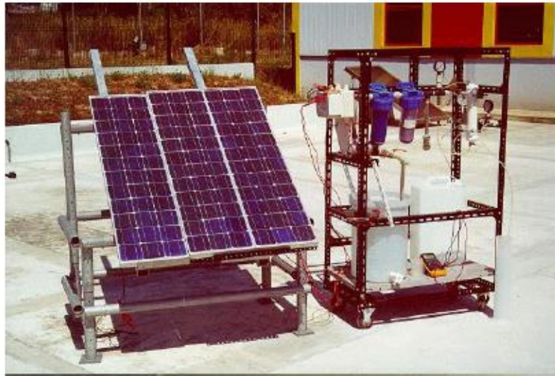
Figure 2.7: Solar water RO system (Chafidz et al., 2016)
