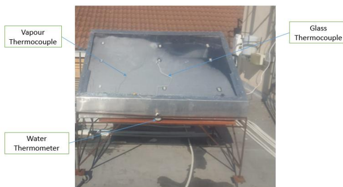
Figure 4.9: Non-tracking (Control) solar water purifier
