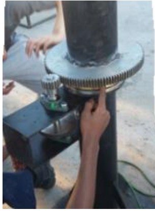
Figure 3.26: Gear alignment and inspection
