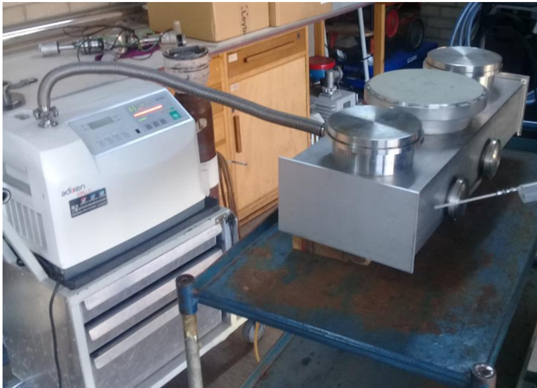
Figure 5.6: Chamber leak testing.
