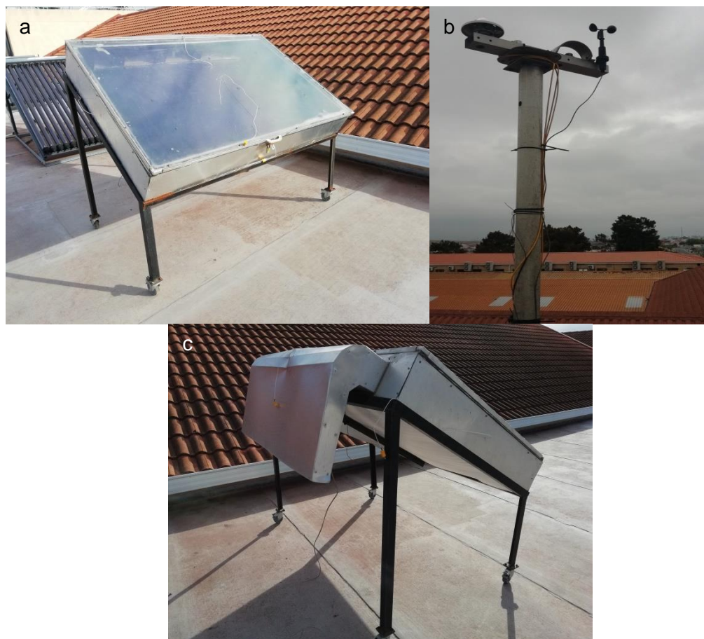
Figure 4.13: (a) Front view of the solar crop dryer model and (b) the weather station (c): Back view of the solar crop dryer
