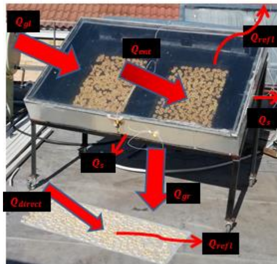
Figure 4.17: Heat transfer in a crop dryer system
