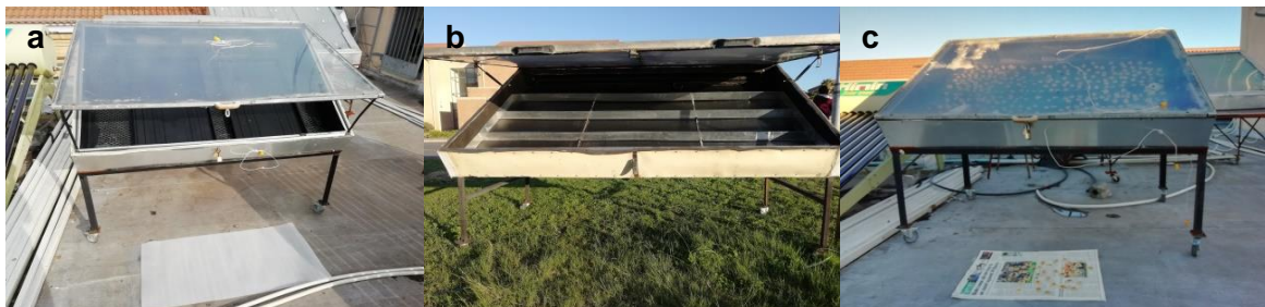
Figure 5.1: Solar crop dryer setup (a) forced extraction dryer (b) natural ventilated dryer and (c) open sun drying
