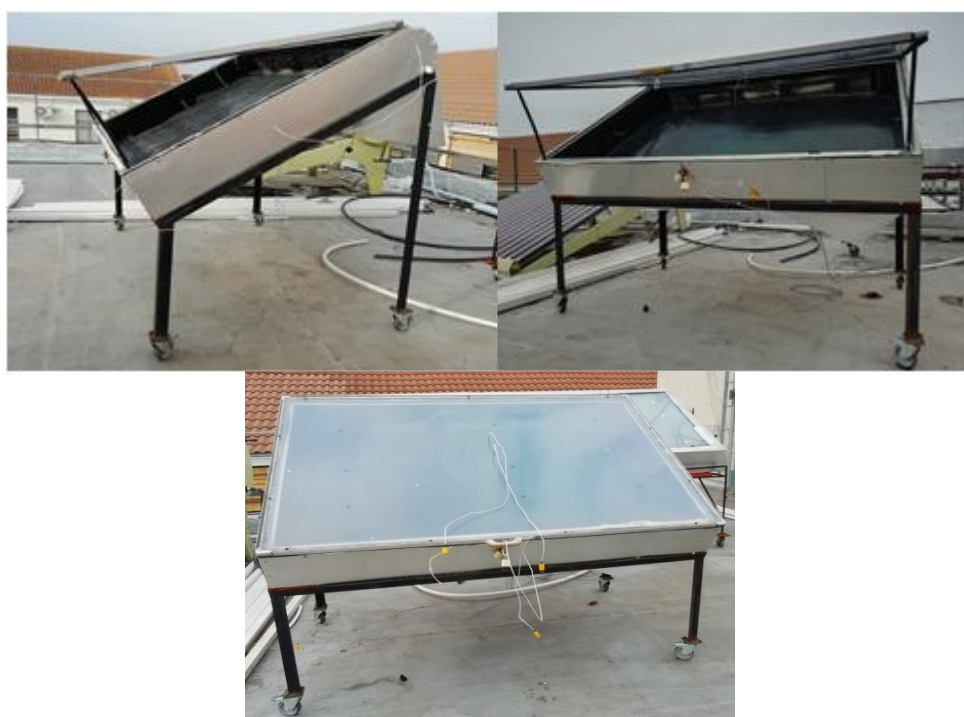
Figure 3.11: Overall dryer design and setup
